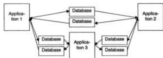
Fig. 1.3. Point-to-point integration of several back-end application systems based on database systems
