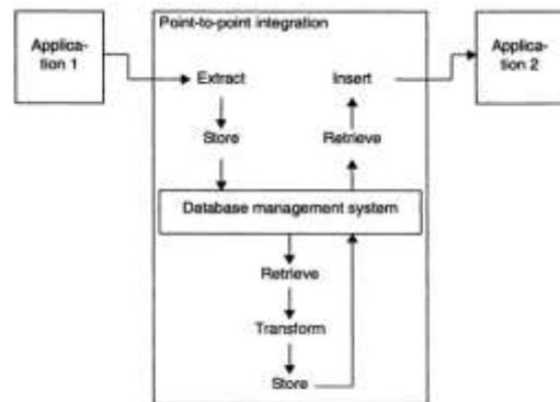
Fig. 1.2. Asynchronous point-to-point integration with a database system as intermediate storage
