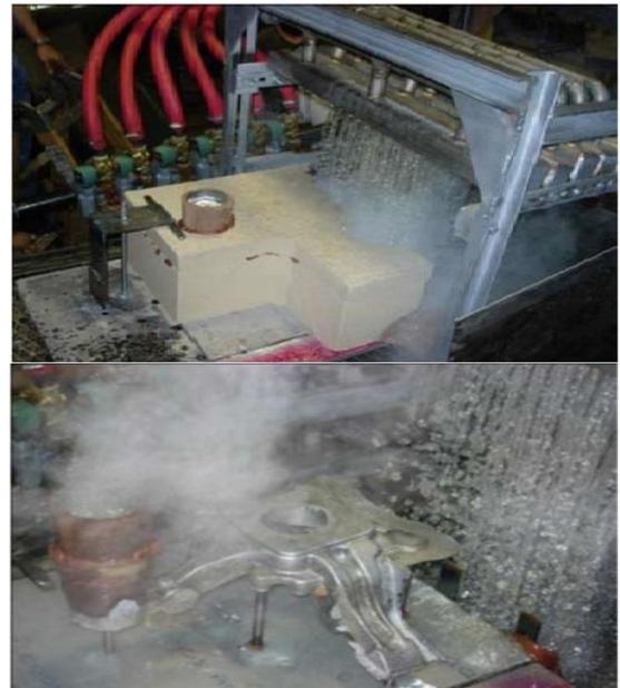
Fig. 1. The execution of the process of ablation casting [2]
