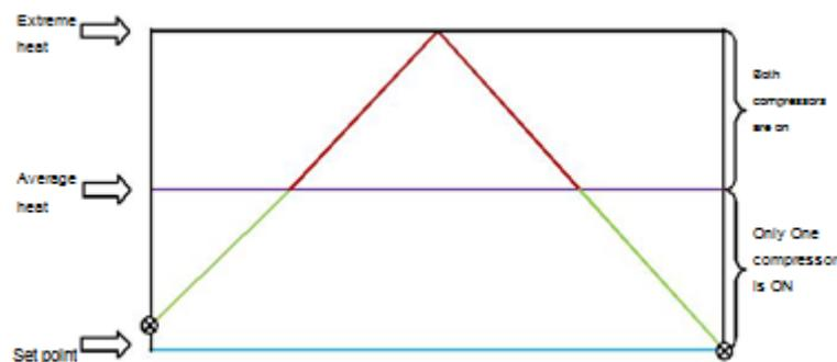
Fig.2 The working principle of two compressor controller
