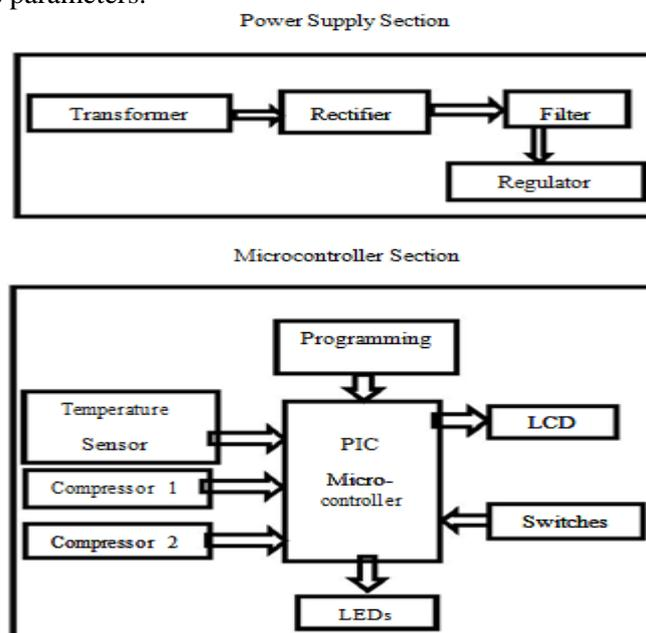
Fig.1 The block diagram of dual compressor controller
