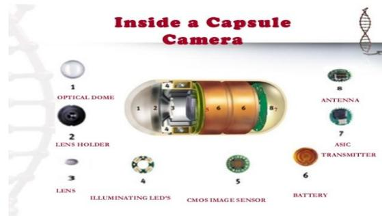
Fig .2 : Structure of Pill Camera
