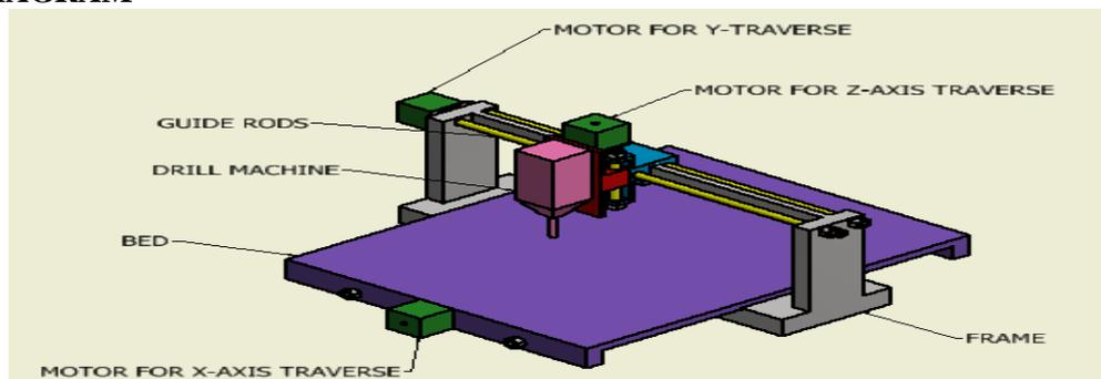
Figure 3.1 Initial Layout of Machine
