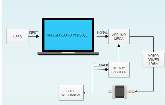
Figure 3.8 Block Diagram of Driving Circuitry
