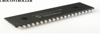
This is the heart of our complete project. It is responsible for all process being executed. It will monitor & control all the comprising devices or components connected in this unit
