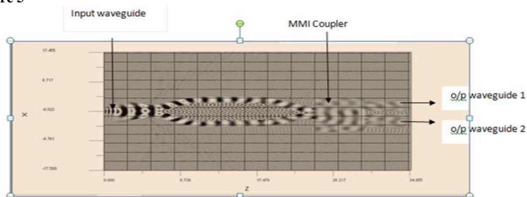
**Fig.4: Propagation of light in the equal arm MZI TTD line**
