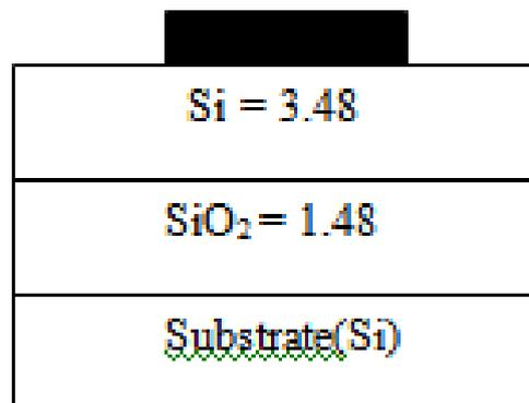
Fig.2: Silica on Silicon Ridge waveguide
