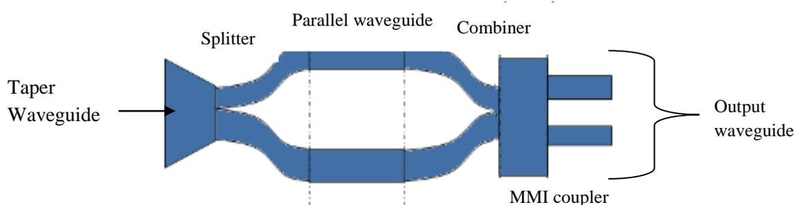
Fig.1: Unequal arm MZI based True Time Delay Line
