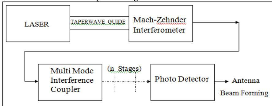
**Fig.3: Simulation set up for antenna beamforming**
