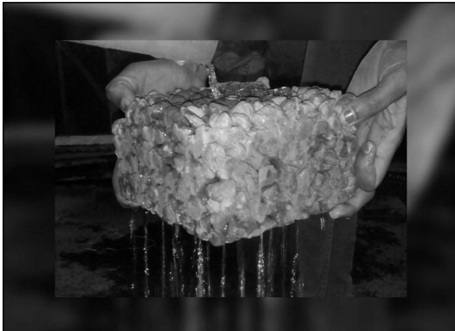
Fig 4.3 porosity test on porous concrete block
