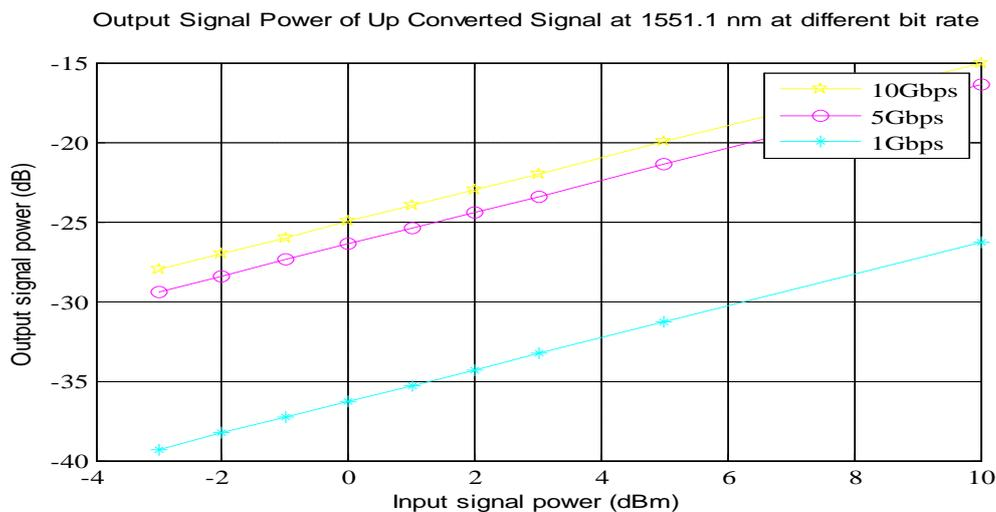
Fig. 6 Output Signal Power of Upconverted signal at 1551.1 nm at different bit rate
