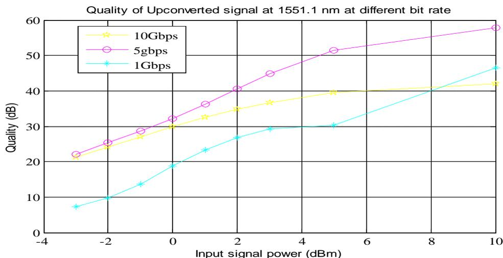
Fig. 4 Quality of Upconverted signal at 1551.1 nm at different bit rate
