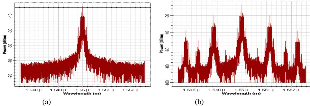
Fig. 3 Optical spectrum of signal after (a) MZM (b) EAM
