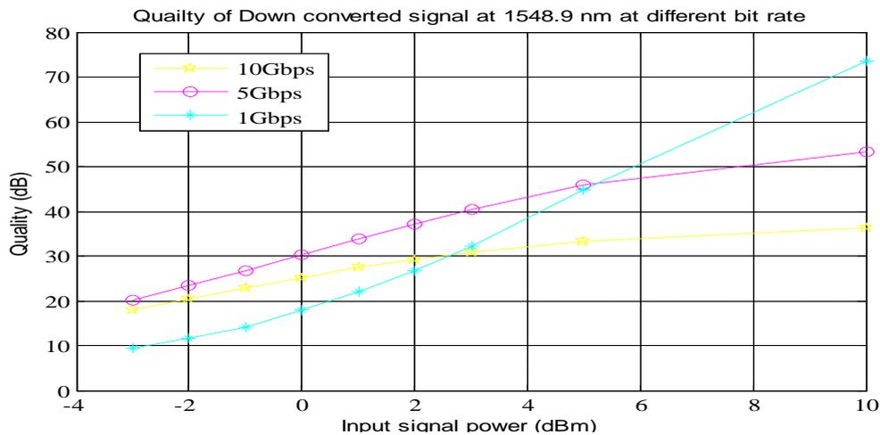
Fig. 5 Quality of Downconverted signal at 1548.9 nm at different bit rate
