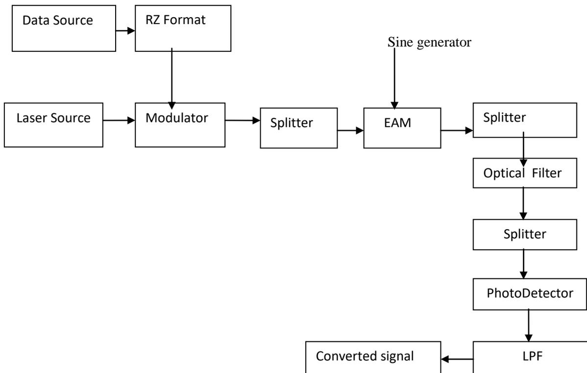
Fig. 1 Schematic Block diagram of RZ format wavelength converter
