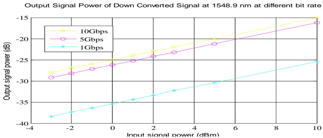
Fig. 7 Output Signal Power of Downconverted signal at 1548.9 nm at different bit rate
