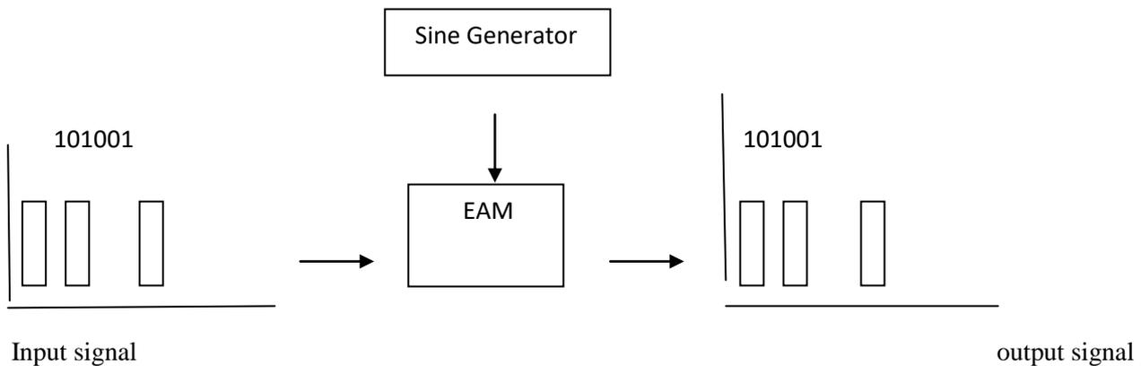
Fig. 2 Basic principle of EAM as wavelength converter
