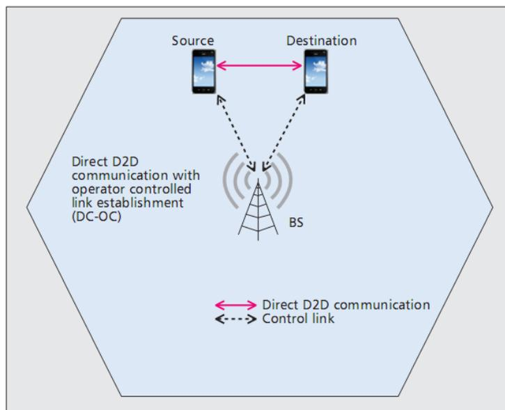
**Fig 2: Direct D2D communication with operator controlled link establishment (DC-OC) [4].**
