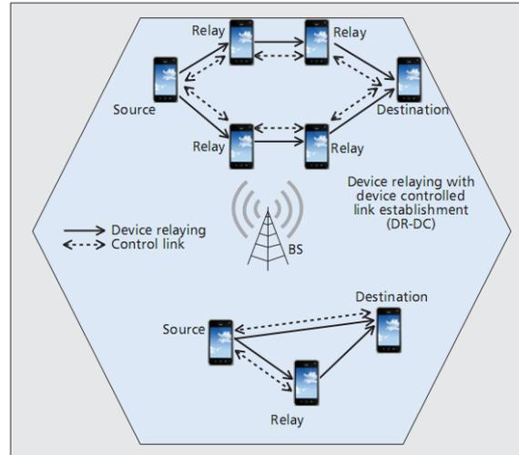
**Fig 3: Device relaying communication with device controlled link establishment (DR-DC) [4].**
