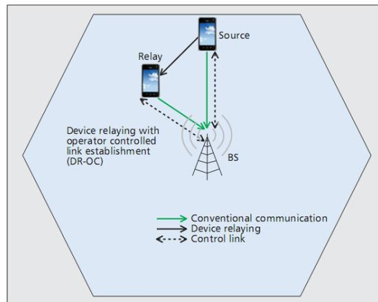
**Fig 1: Device relaying communication with operator controlled link establishment (DR-OC) [4].**
