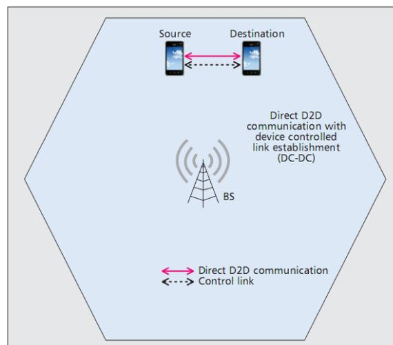
**Fig 4: Direct D2D communication with device controlled link establishment (DC-DC) [4].**
