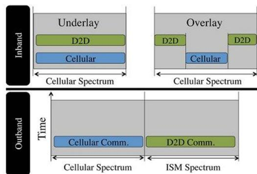
**Fig 6: Representation of underlay inband, overlay inband and outband D2D [6].**
