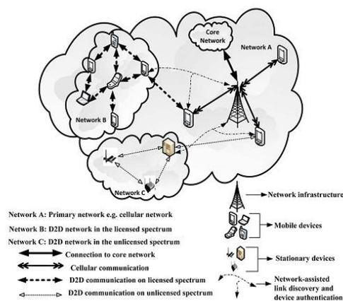
**Fig 8: Network-infrastructure-dependent D2D communication using a licensed or an unlicensed frequency spectrum [3].**
