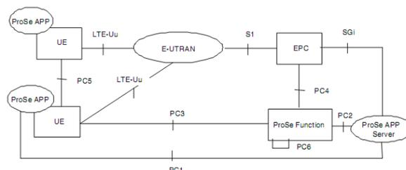
**Fig7: D2D enhanced LTE architecture [13]**
