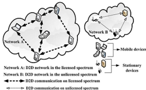
**Fig.9. Network-independent D2D communication using a licensed or an unlicensed frequency spectrum [3].**
