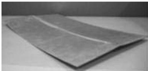
Fig.7. Distortion – TIG (Yan Dong-yang et al, 2010)
