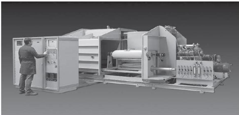
**Figure:-** Large industrial roll-to-roll vacuum plasma treatment machine
