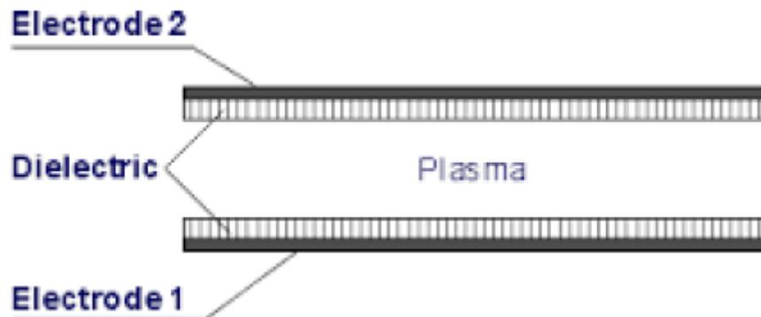
**Figure:-** Dielectric barrier discharge
