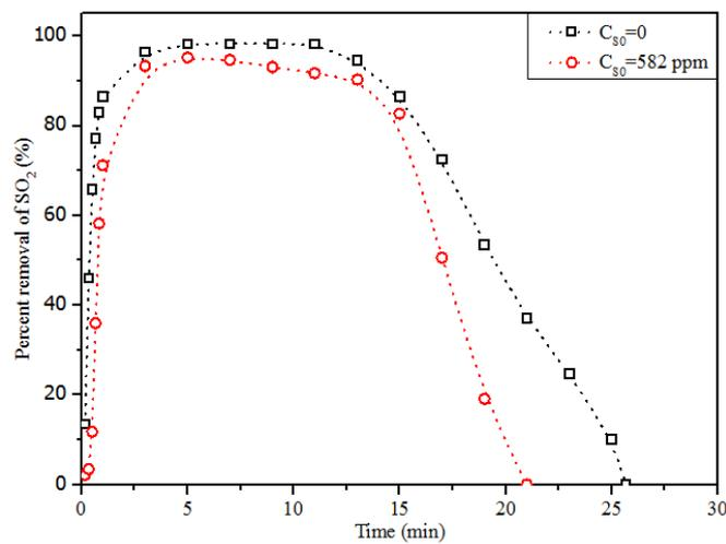
Figure 2 Percent removal of SO<sub>2</sub> in bubble column with/without surface active agent
