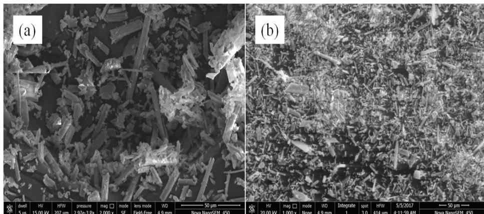
**Figure 5 SEM image of FGD product obtained by (a) bubble column (without surface active) and (b) foam-bed reactor (in presence of surface active agent, Triton X-100)**
