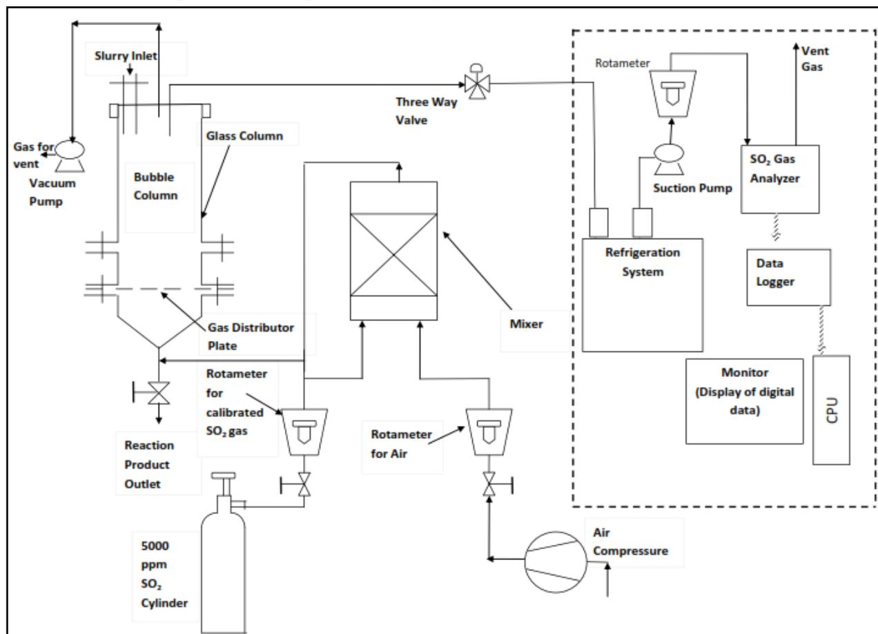
Figure 1 Line diagram for SO<sub>2</sub> absorption apparatus
