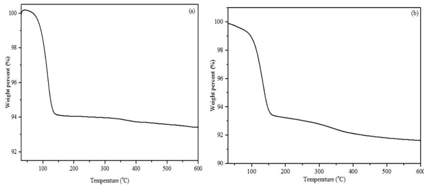
**Figure 4 TGA analysis of FGD product obtained by (a) bubble column (without surface active) and (b) foam-bed reactor (in presence of surface active agent, Triton X-100)**
