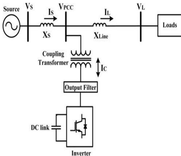
Fig. 1 Schematic diagram of DSTATCOM
