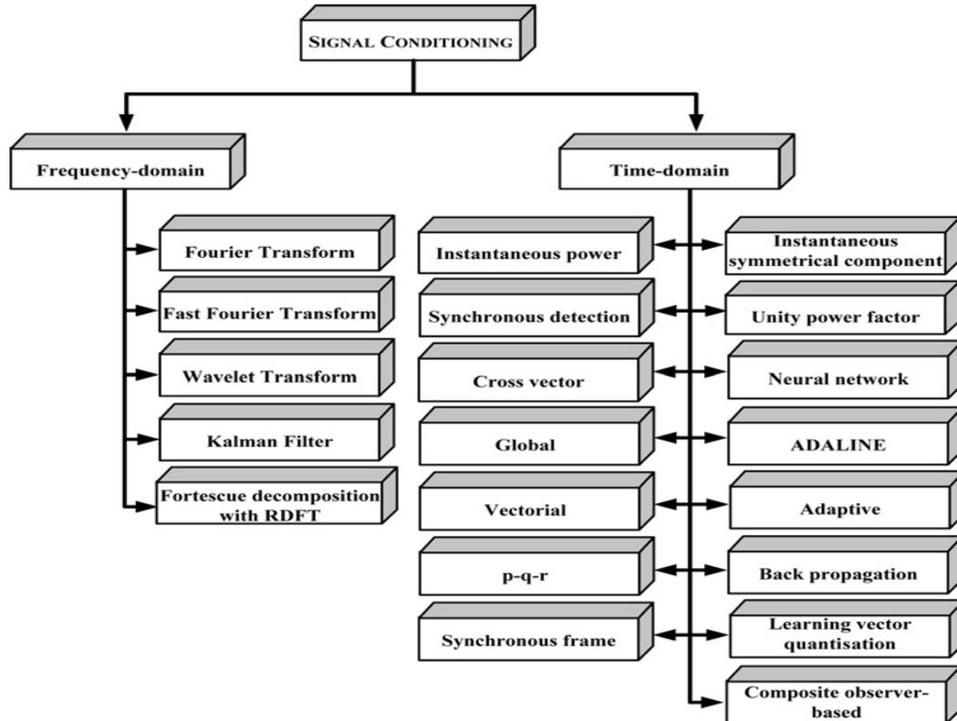
Fig.5 Classification according to reference signal extraction techniques [33]
