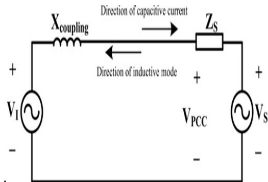
Fig. 2 Equivalent circuit of a single-phase power system with a DSTATCOM [33]
