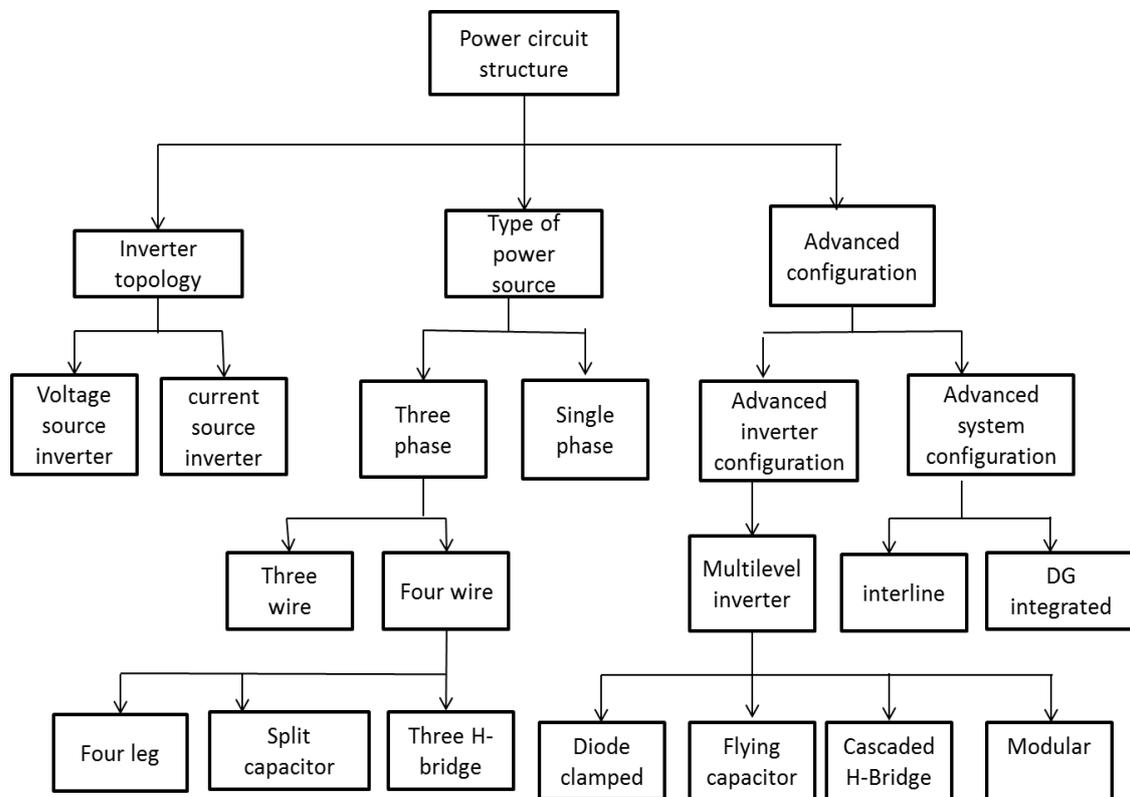
Fig 4 Classification of DSTATCOM based on power circuit structures [33]
