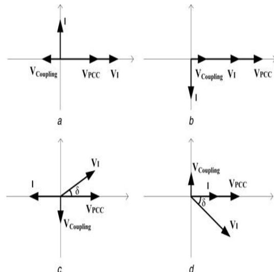
Fig. 3 Vector diagrams of DSTATCOM[33]
