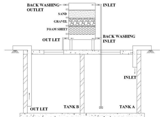
FIG. 2 (e) storage tank & filtration unit
