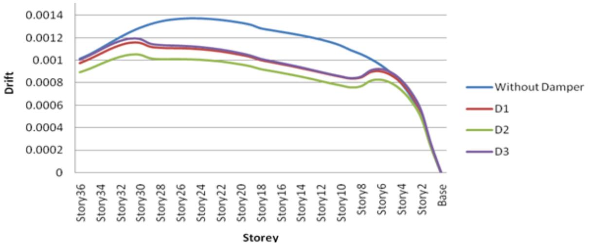
**Figure 5: Storey drift response of structure in X-direction (SpecX)**
