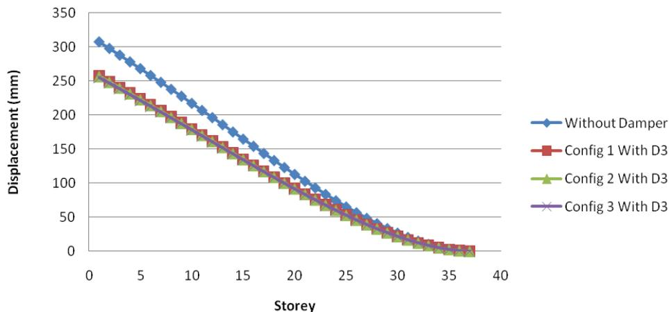
**Figure 3: Displacement Due to Wind Y in Y Direction for Various Configurations**
