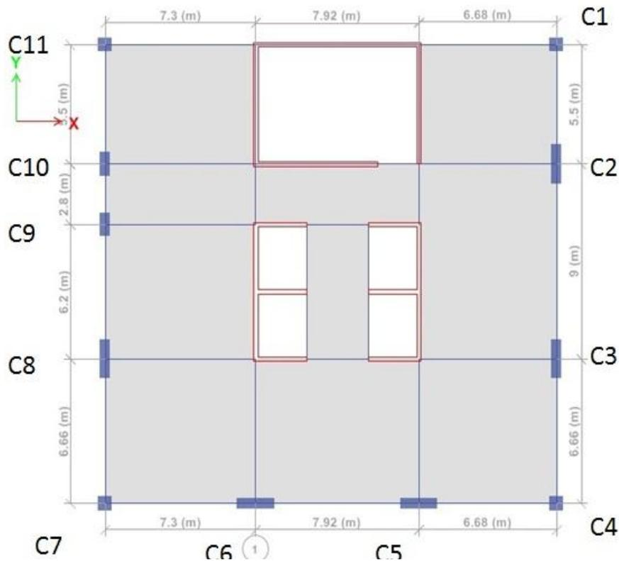
**Figure 1: Typical Plan of G+35 RCC Building**
