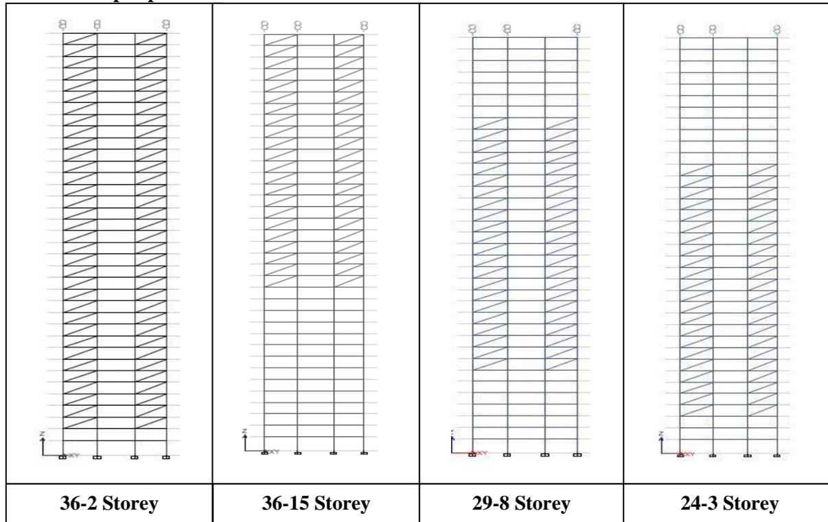
**Figure 4: Various Damper Placement Locations**
