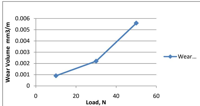
**Figure- 5: Wear volume increasing with increasing load**
