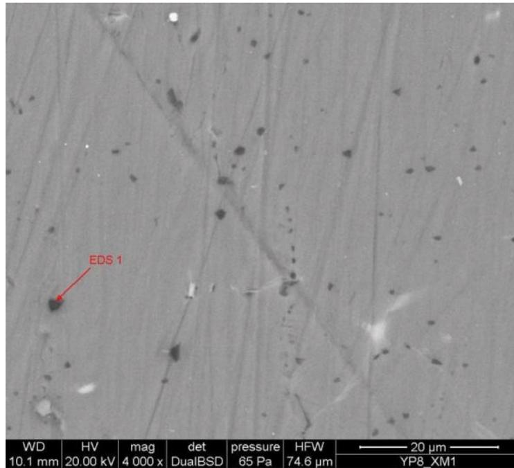
**Figure-3: Uniform reinforcement of B4C & Ni80Cr20 particles in coating.**
