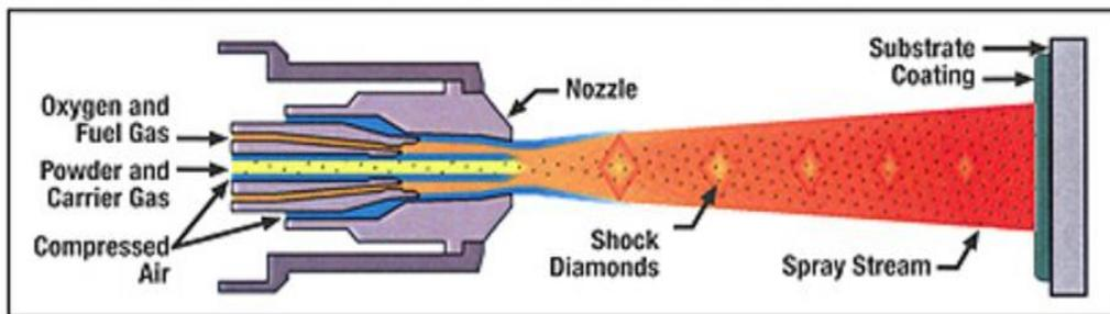
**Figure-1: Principle of HVOF process (Courtesy: Eastern Metallizing Co Pvt Ltd, Kolkata)**
