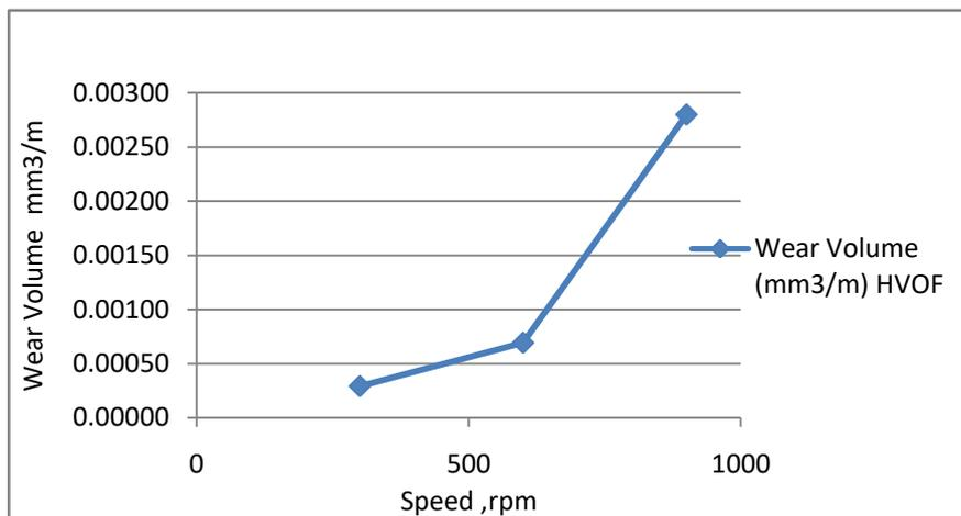
**Figure-6: Wear volume increasing with increasing Speed.**
