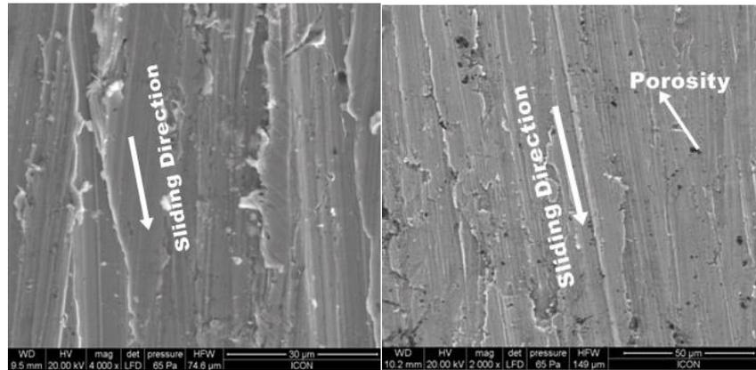
**Figure- 8:Worn surface & sliding direction of wear with increase in load.**
