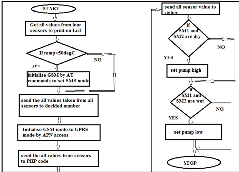
**Figure 5 Transmitter flowchart**
