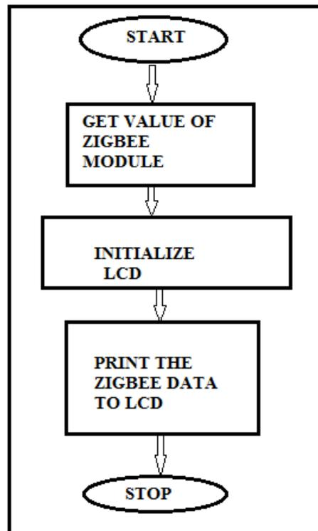
**Figure 6. Receiver flowchart**
