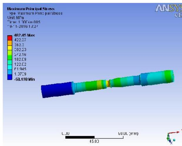
Figure 4.2: ANSYS Analysis of Bar with U Notch 1.5mm Depth
