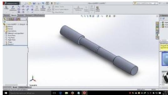
**Figure 3.5: Bar with V Notch 1.5mm depth**
