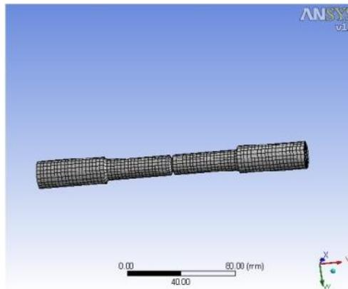
**Figure 3.12: Mesh (Bar with V Notch 3mm depth)**
