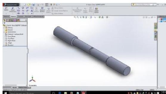
**Figure 3.8: Bar with U Notch 3mm depth**
