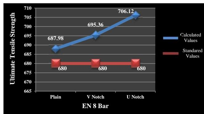
Figure 4.11: Notch effect on Tensile Strength of Bar (9mm dia)
