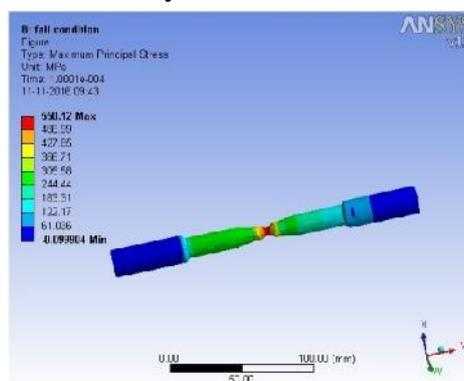
Figure 4.9: ANSYS Analysis of Bar with V Notch 3mm Depth
