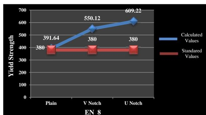
Figure 4.12: Notch effect on Yield Strength of Bar (9mm dia)
