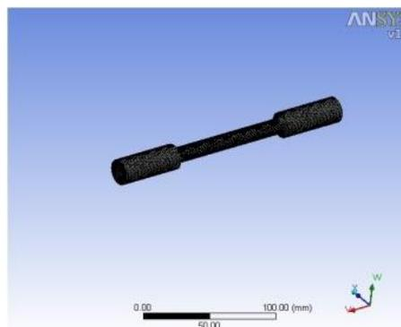
**Figure 3.10: Mesh (Plain Bar of 12mm Dia)**
