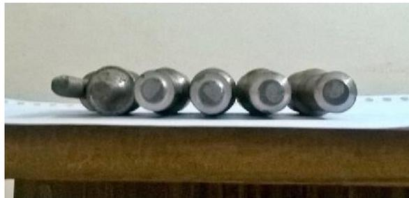
Figure 4.7: Specimen after Tensile Testing from UTM (9mm)
