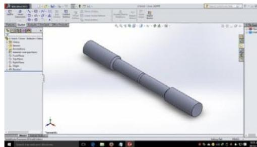
**Figure 3.7: Bar with U Notch 1.5mm depth**
