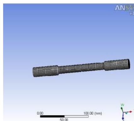
**Figure 3.11: Mesh (Bar with V Notch 1.5mm depth)**
