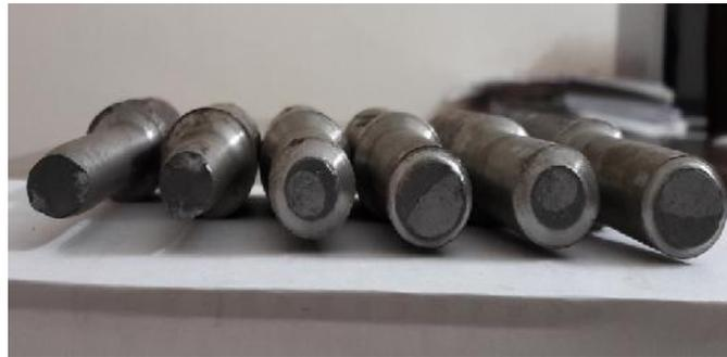
Figure 4.1: Specimen after Tensile Testing on UTM (12mm)
