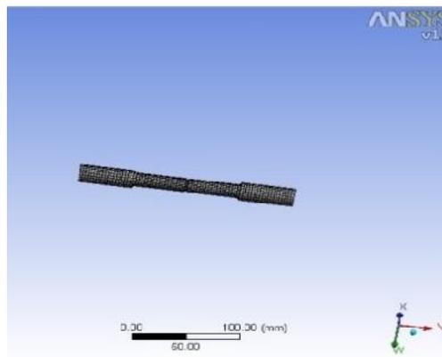
**Figure 3.13: Mesh (Bar with U Notch 1.5mm depth)**
