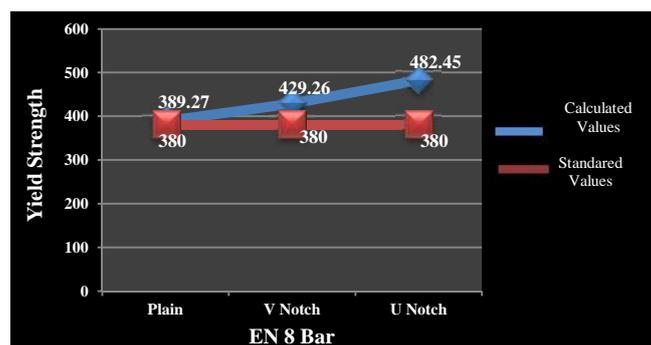
Figure 4.6: Notch Effect on Yield Strength of Bar (12mm Dia.)
