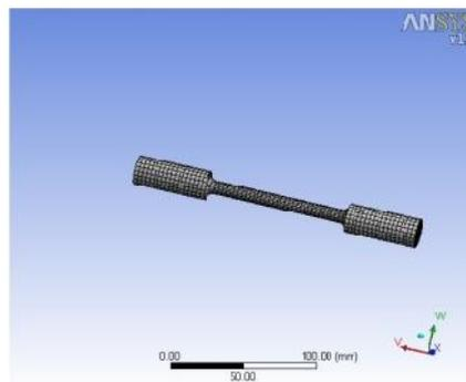
**Figure 3.9: Mesh (Plain Bar of 9mm Dia)**
