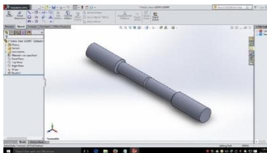
**Figure 3.6: Bar with V Notch 3mm depth**
