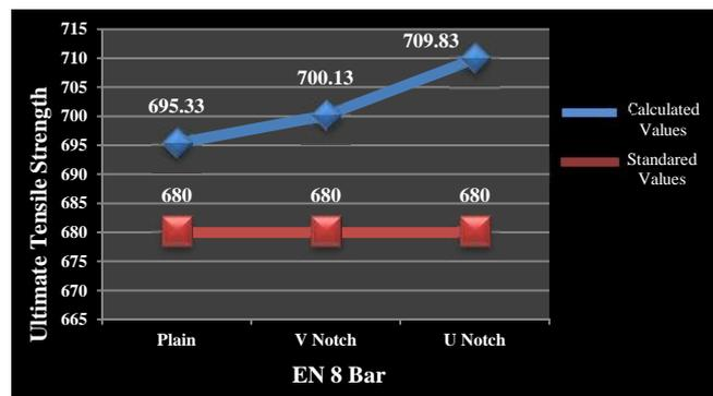
Figure 4.5: Notch Effect on Ultimate Tensile Strength of Bar (12mm Dia.)
