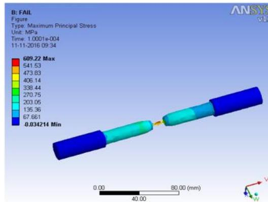
Figure 4.8: ANSYS Analysis of Bar with U Notch 3mm Depth
