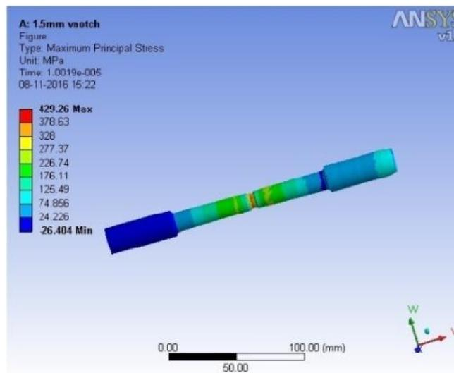
Figure 4.3: ANSYS Analysis of Bar with V Notch 1.5mm Depth
