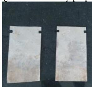
**Fig 2: Aluminium Electrodes**
