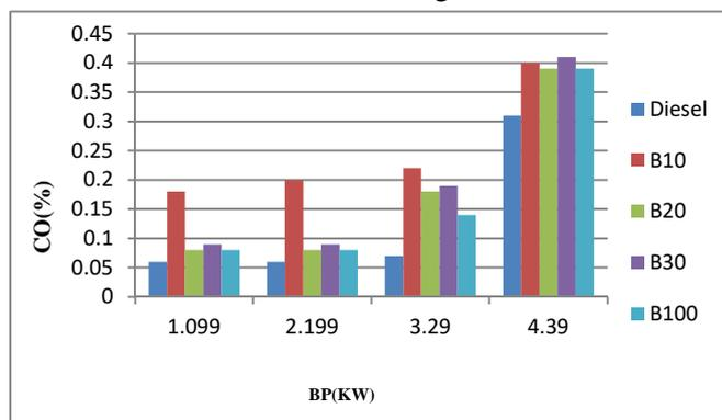
**Graph1.12 SHOWS CO (CARBON MONOXIDE) V/S BP (BRAKE POWER) FOR DIESEL AND PONGAMIA AND COTTON SEED OIL BIO-DIESELS BLENDS**
