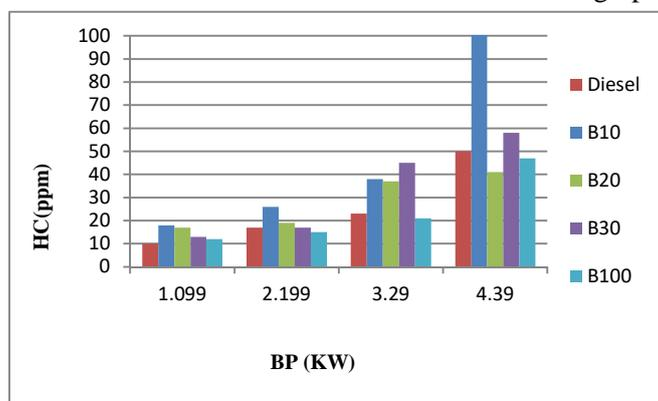
**Graph 1.11 HC (HYDROCARBON) V/S BP (BRAKE POWER) FOR DIESEL AND PONGAMIA AND COTTON SEED OIL BIO-DIESELS BLENDS**
