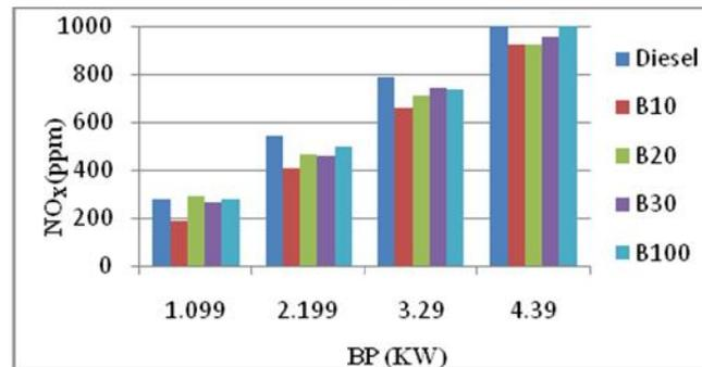
**Graph 1.13 NO<sub>x</sub> (NITROGEN OXIDE) V/S BP (BRAKE POWER) FOR DIESEL AND PONGAMIA AND COTTON SEED OIL BIO-DIESELS BLENDS**
