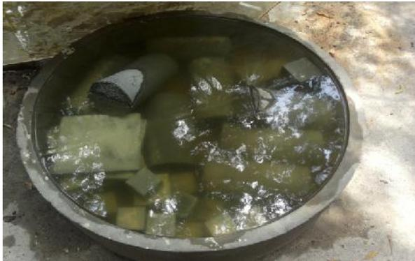
**Fig 1: Curing of Specimen in Water**
