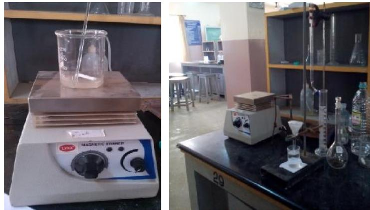
**Fig 8: Sample placed in magnetic stirrer and filtration of solution**
