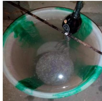
**Fig 4: Specimens kept in Hot Water**
