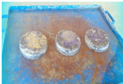
**Fig 6: Specimens kept in Water for curing**
