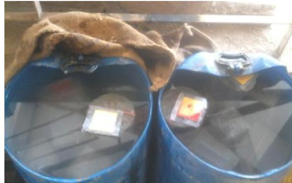
**Fig 2: Curing of Specimen in NaCl Solution**
