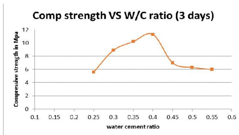
Fig-3 Compressive strength in Mpa VS water cement ratio for 3 days
