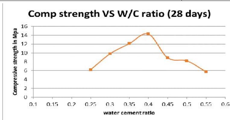
Fig-5 Compressive strength in Mpa VS water cement ratio for 28 days
