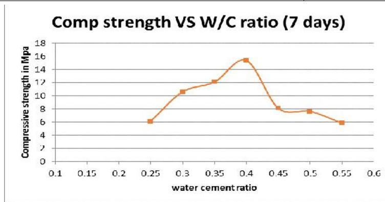
Fig-4 Compressive strength in Mpa VS water cement ratio for 7 days
