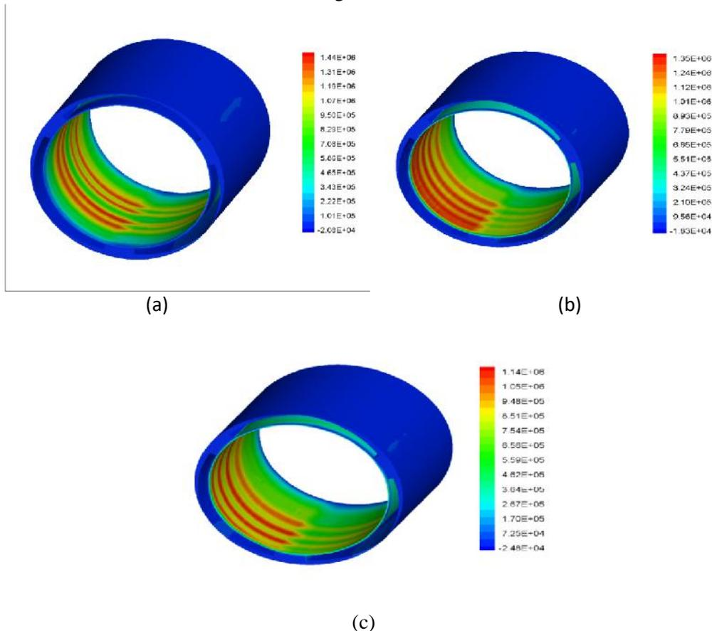
**Fig. 5.5 Contours (a), (b), (c) are Total Pressure contours for ISO-VG-46, SAE-50 and SERVO PRIME-46 oil respectively.**
