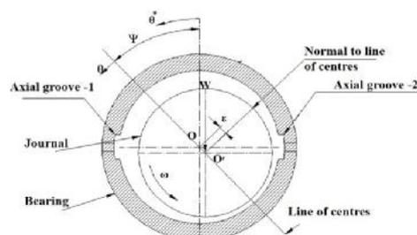
**Fig. 1.1 Axial Grooved Bearing [5]**
