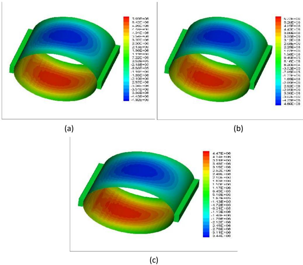
**Fig. 5.1** Contours (a), (b), (c) are Total Pressure contours for ISO-VG-46, SAE-50 and SERVO PRIME-46 oil respectively.
