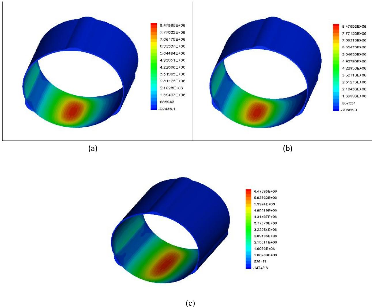
**Fig. 5.3** Contours (a), (b), (c) are Total Pressure contours for ISO-VG-46, SAE-50 and SERVO PRIME-46 oil respectively.
