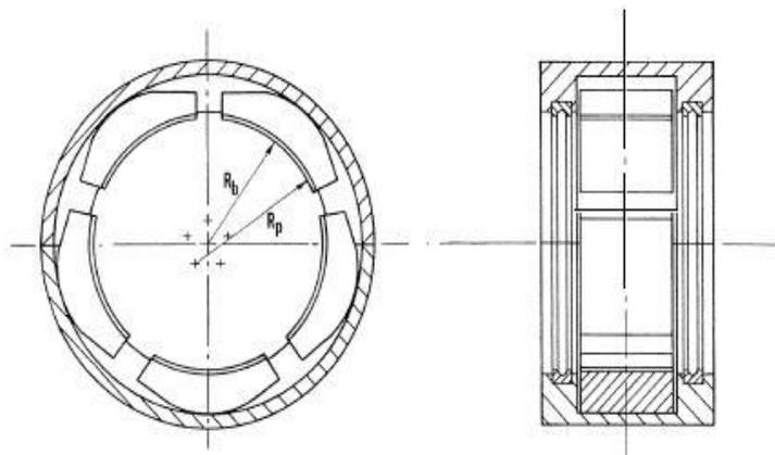
**Fig. 1.3 Tilting Pad Bearing [9]**
