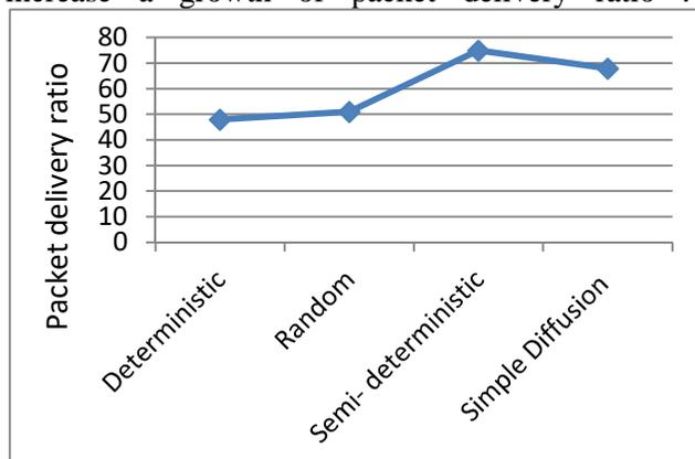
**Figure 7. Packet Delivery ratio for various node placement**
