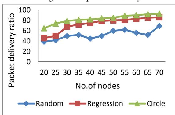
**Figure 8. Packet Delivery ratio for various node placement methodology**
