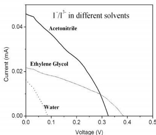
**Fig 2: V-I graph of different solvents for  $\text{I}^-/\text{I}_3^-$  electrolyte based DSSC**
