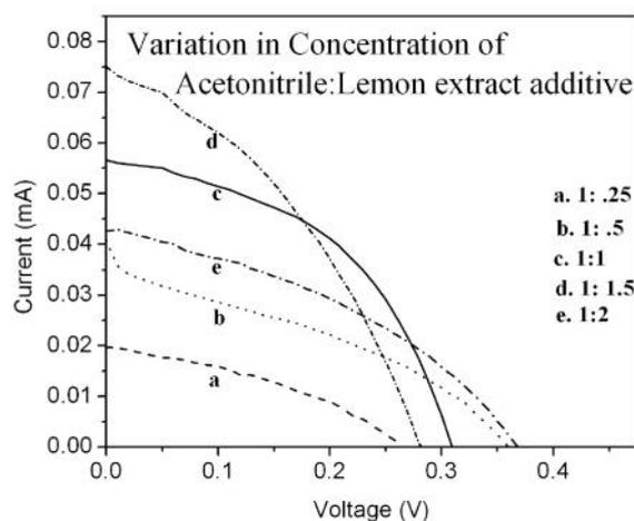
**Fig 5: V-I graph of cells with various volume ratio of acetonitrile and lemon extract**
