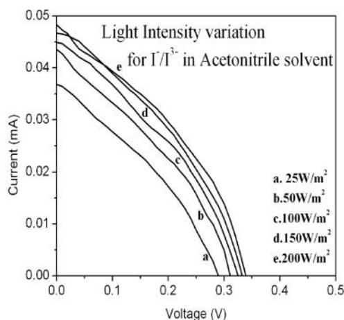
Fig 3: V-I graph of DSSC showing the effect of intensity variation on  $I/I^3$ -electrolyte in acetonitrile solvent
