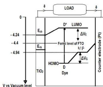
**Fig 1: Energy level diagram of DSSC**
