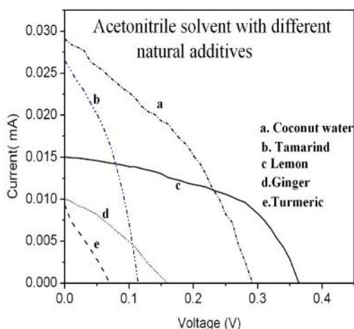
Fig 4: V-I graph of DSSC in acetonitrile solvent with different natural additives
