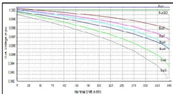
Fig. 8. The PV curve for 110% loading with SVC device in PWS
