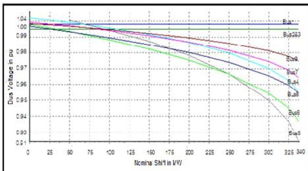
Fig. 7. The PV curve for 110% loading without SVC device in PWS
