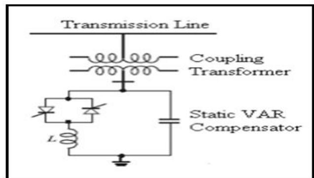
Fig. 1. Schematic Diagram of FC-TCR
