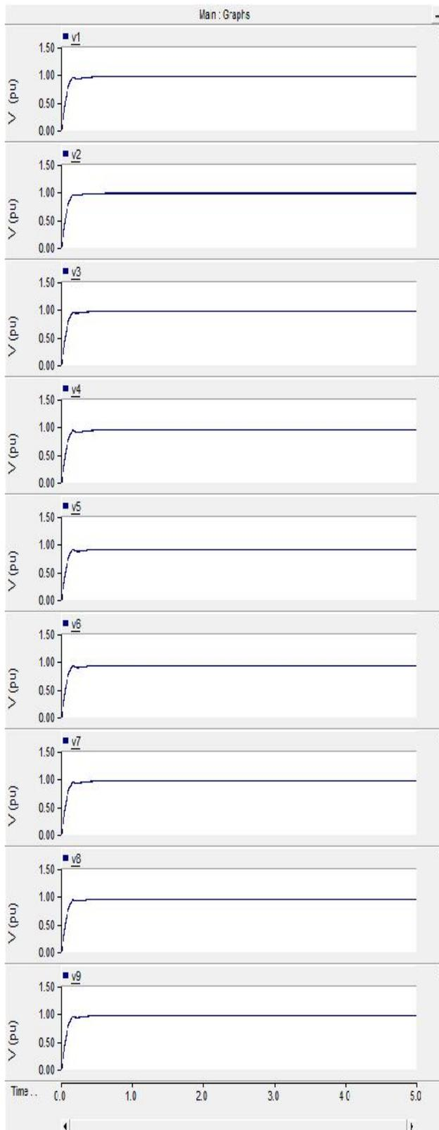
Fig. 5. Voltage waveform of each bus at 110% loading without SVC
