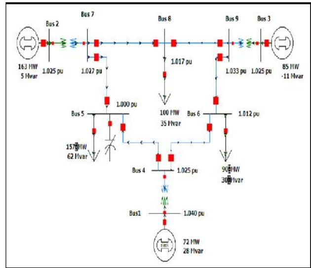
Fig. 4. Simulated Circuit of IEEE 9 BUS SYSTEM in PWS [3]
