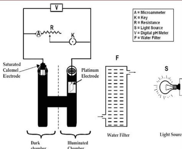
Figure 1: Experimental set up of photogalvanic cell
