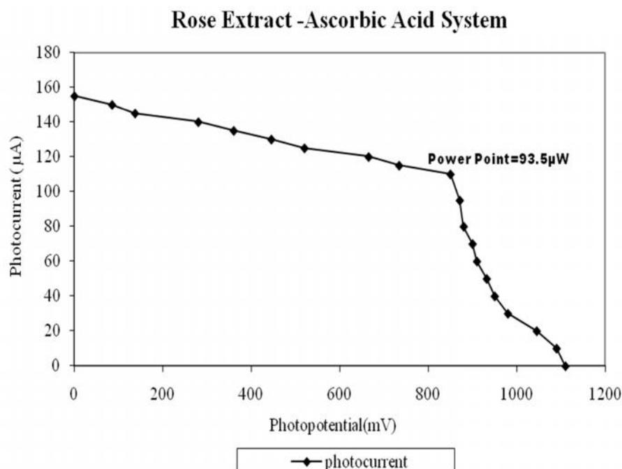
**Figure 4: Current-potential (i-V characteristics) of the Cell**
