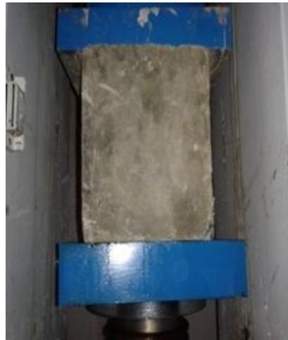
**Figure.5. Testing for Compressive strength**
