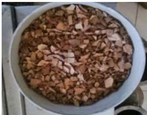
**Figure 1. Coconut shell aggregate**
