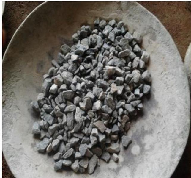
**Figure 2. Crushed stone aggregate**
