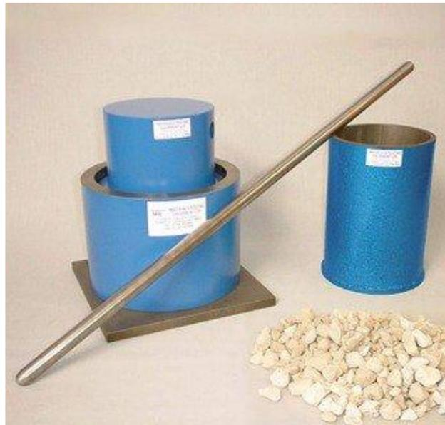
**Fig.3.Aggregate crushing strength Test**
