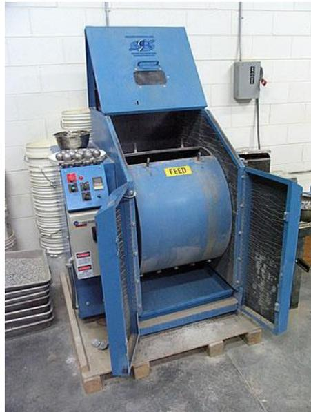
**Fig.4. Los Angel Abrasion Test**
