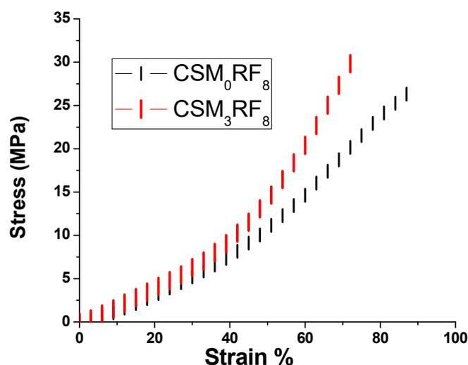
**Figure 2: Plot of Mechanical Properties of the samples  $\text{CSM}_0\text{RF}_8$  and  $\text{CSM}_3\text{RF}_8$**
