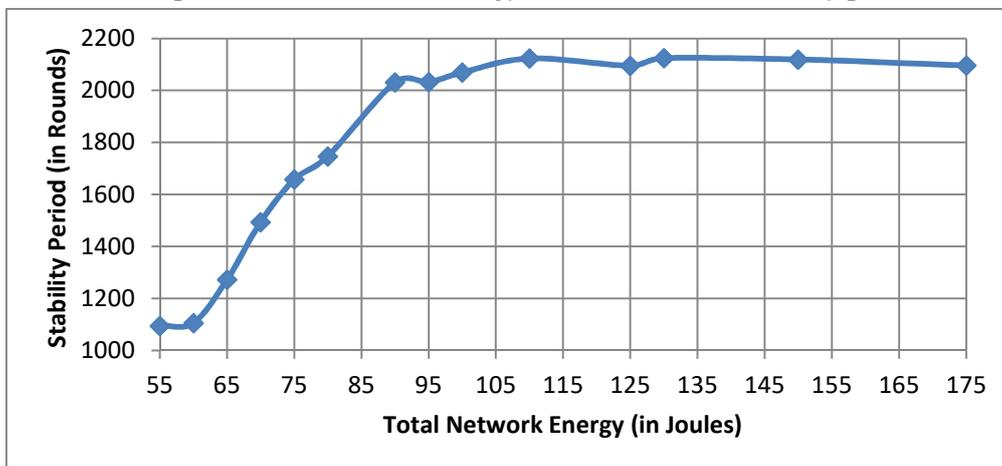
**Fig 1: Total Network Energy vs Stability Period**
