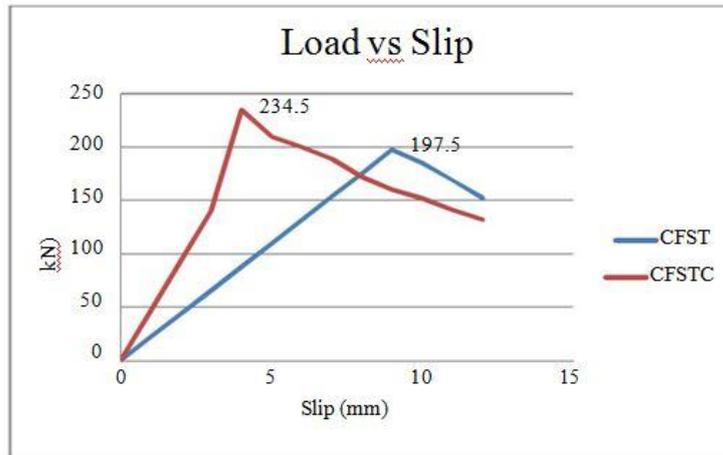
Figure.6 Failure load
