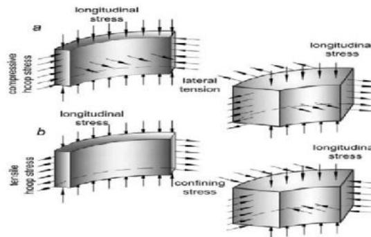
Figure.1 Stress condition in steel tube and concrete core at different stages of loading
