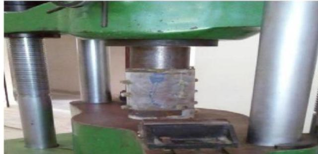
Figure .4a Experimental setup for push out test
