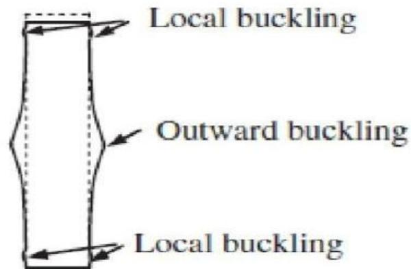
Figure.9 Failure Pattern
