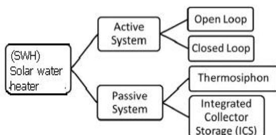
Fig: 5 Categories of Solar water heating system (SWH)
