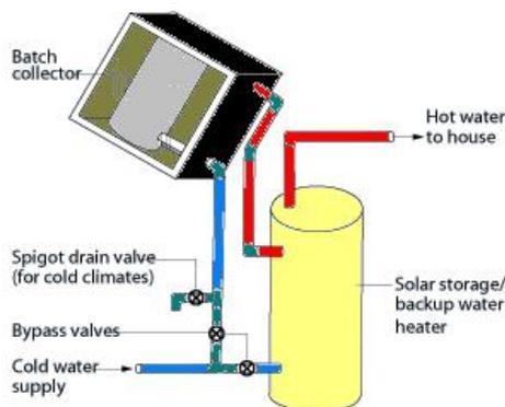
Fig: 7 Passive Solar water heating system
