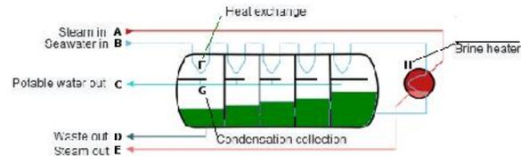
Fig: 3 Schematic layout of Multi Stage Flash
