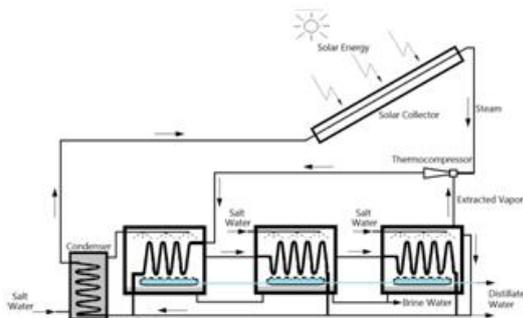
Fig: 2 Schematic layout of Multi effect distillation.
