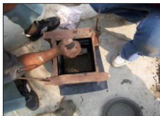
**Fig.7: COMPACTING OF MIXTURE**
