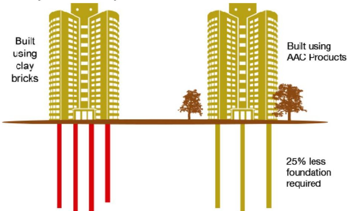
**Fig.11: FOUNDATION DEPTH LESS AS COMPARED TO BRICKS**
