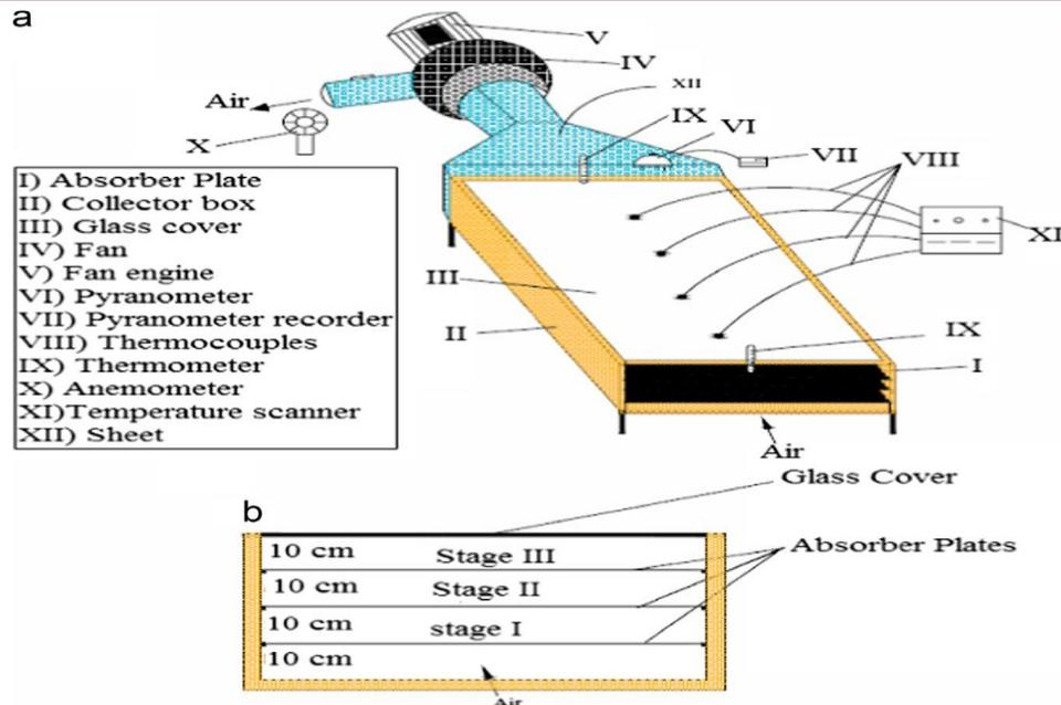
Fig. 3. Schematic assembly of the (a) SAH system and (b) front view of the collector
