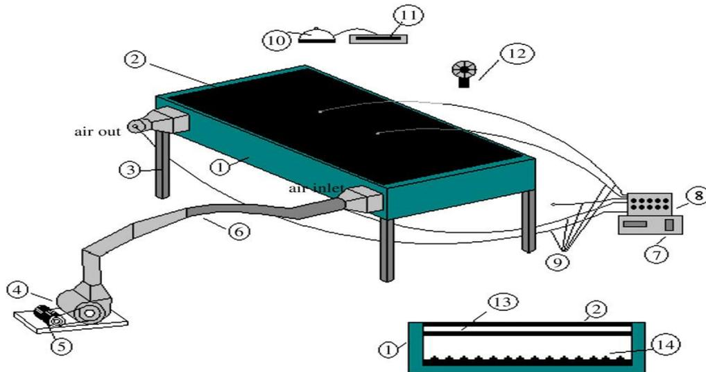
Fig. 2. Schematic view of experimental set-up: 1) Collector Box 2) Glass Cover 3) Foot 4) Fan 5) Fan Engine 6) Connection Pipe 7) Channel Selector 8) Digital Thermometer 9) Thermocouples 10) Pyranometer 11) Pyranometer recorder 12) Anemometer 13) Absorber plate (copper plate that's been painted black) 14) Absorber plate with (Different) obstacles as reported by Ref.[20].
