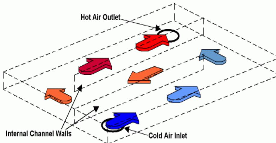
Fig. 1 A typical Solar Air Heater with Flat Plate Collector
