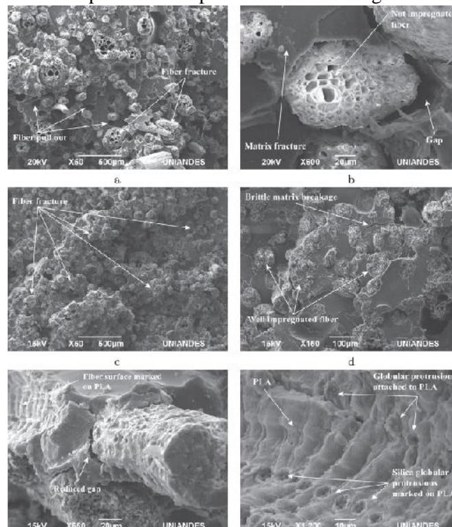
Fig. 3. SEM micrographs of tensile fractured surface. (a and b) Untreated fabric composite and (c-f) optimized composite.
