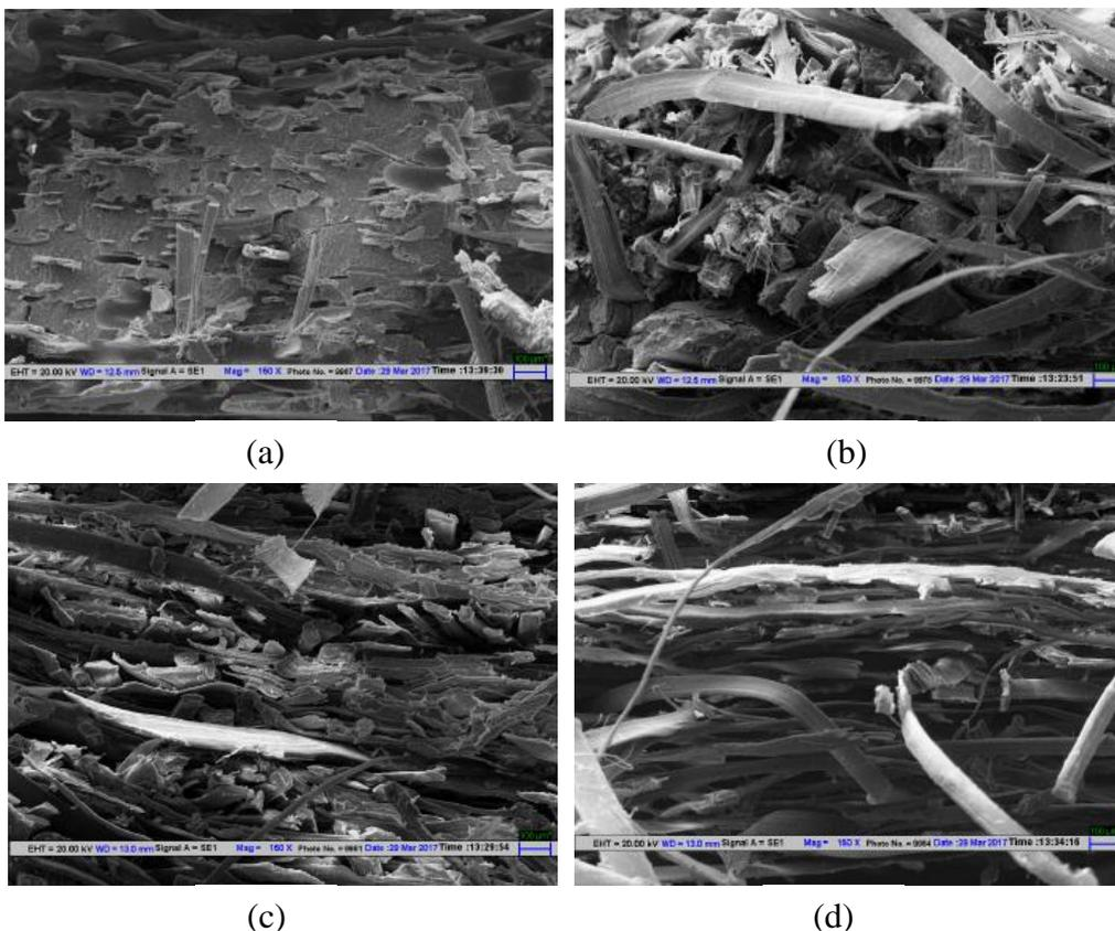
Fig. 1. SEM images of cryo-fractured biocomposites prepared with (a) 10 wt % (b) 25 wt% (c) 50 wt% (d) 75 wt% nettle fibers
