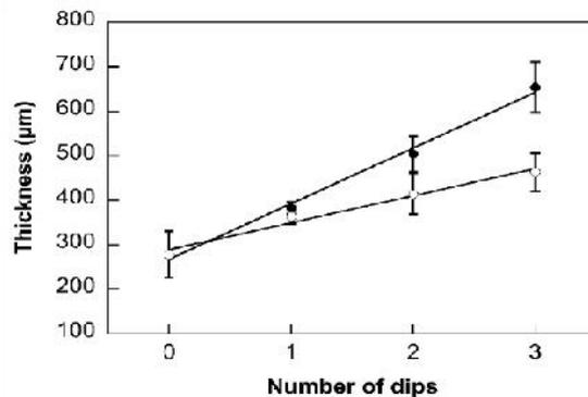
Fig. 2. The sample thickness as a function of the number of dips using the horizontal ( ) and vertical ( ) methods.
