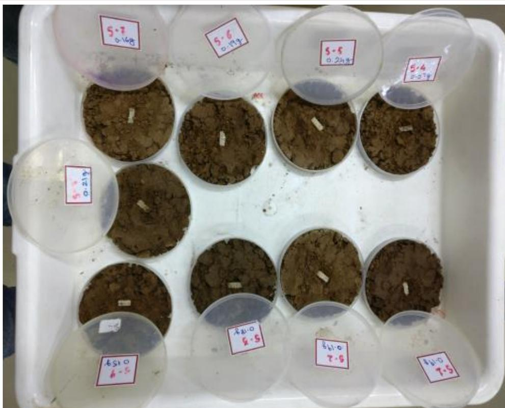
**Fig 10: Samples buried in soil**
