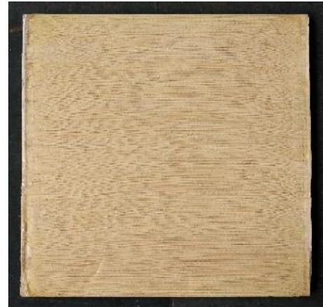
**Fig 7: Fabricated Cotton/Polyester Composite Plate**
