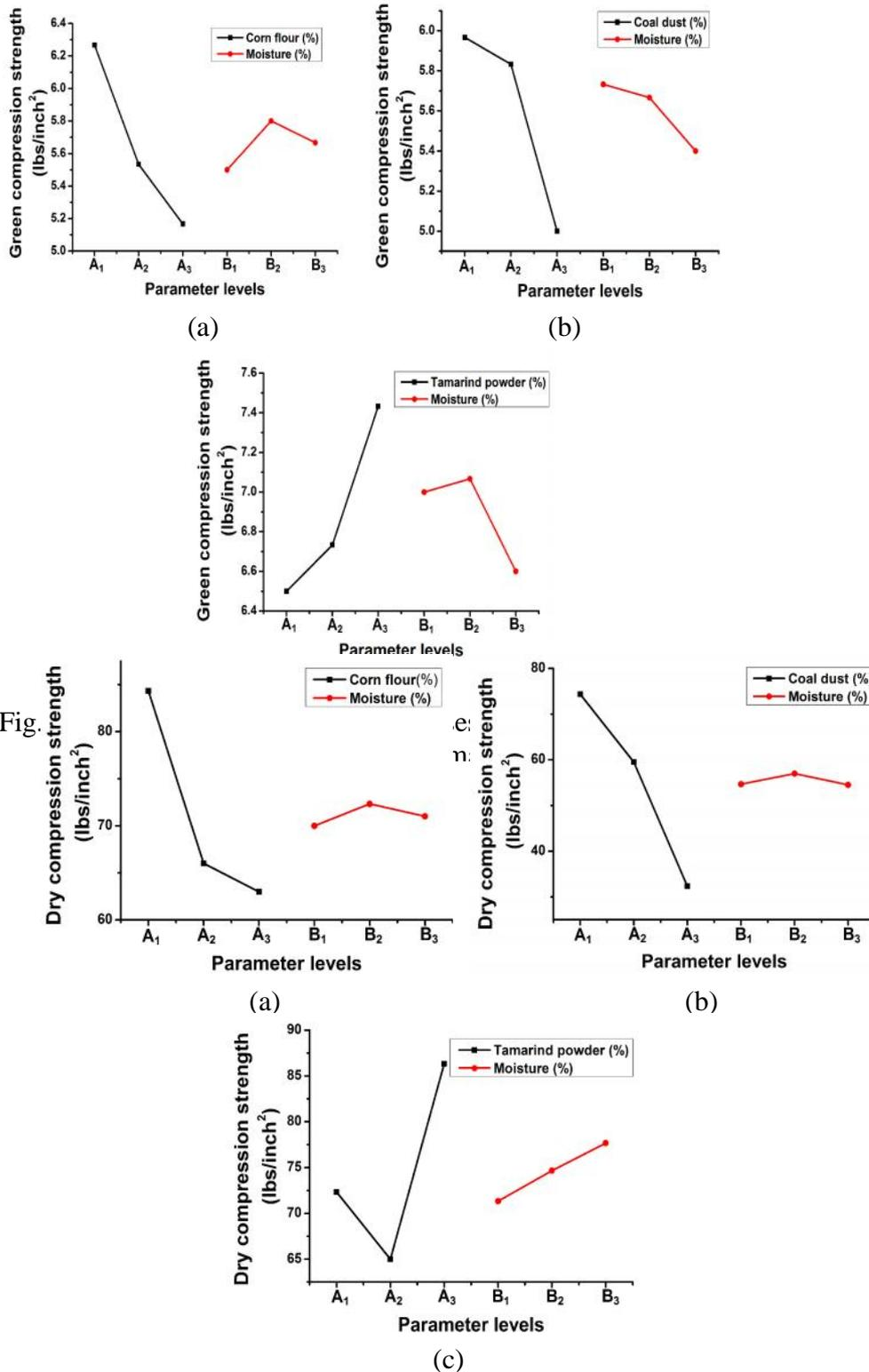
Fig. 4. Dry compression strength versus Parameter levels (a) Corn flour (b) Coal dust (c) Tamarind powder
