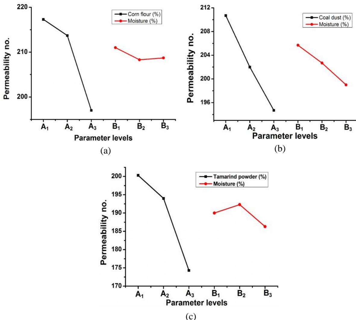
Fig. 2. Permeability no. verses Parameter levels (a) Corn flour (b) Coal dust (c) Tamarind powder
