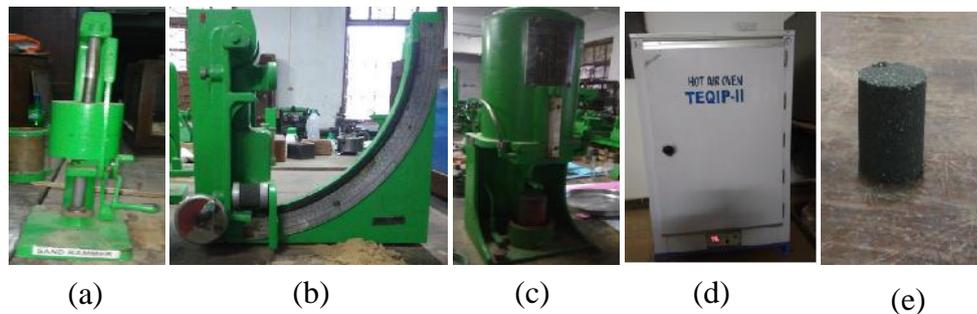
Fig. 1. (a) Sand rammer (b) Universal testing machine (c) Permeability meter (d) Hot air oven (e) Standard test specimen
