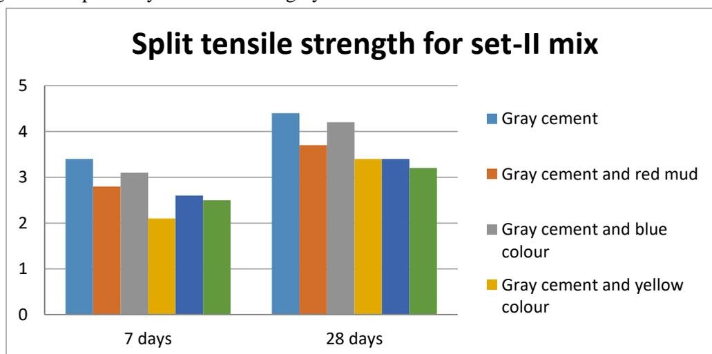
Fig 7: Split tensile strength results for mix design-II
