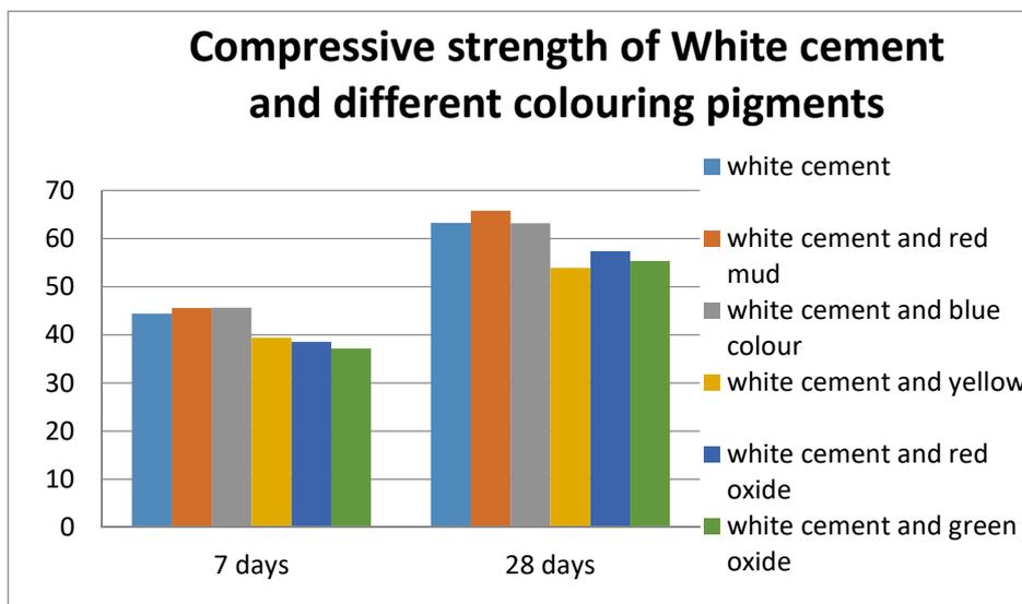
**Fig 4: Compressive Strength of White Cement and Different Pigments (Mix SET-I)**
