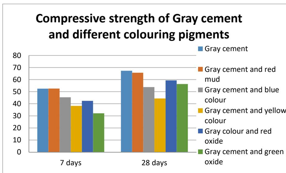
**Fig 5 :Compression Test of OPC Cement and Different Pigments (mix SET-II)**
