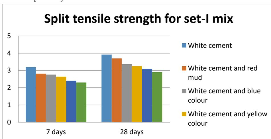
Fig 6: Split tensile strength results for set-I mix
