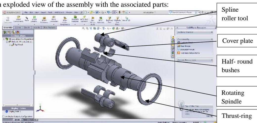
**Fig. 2 Exploded view of the assembly**
