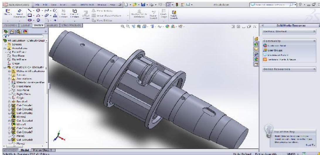
**Fig. 1 3D model of the assembly used for analysis**
