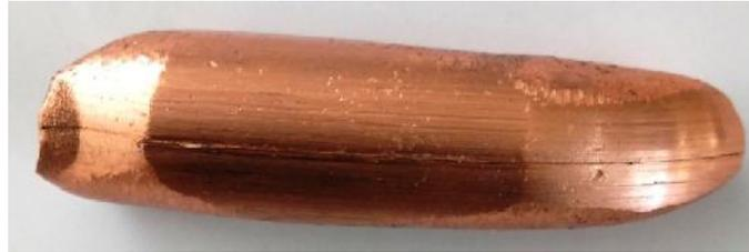
Figure-4: Copper billet after six passes
