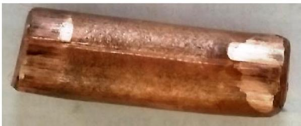
Figure-2: Copper billet after two passes
