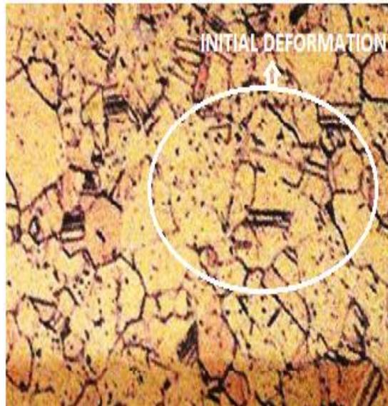
Figure-7: Microstructure after two passes
