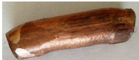
Figure-3: Copper billet after four passes
