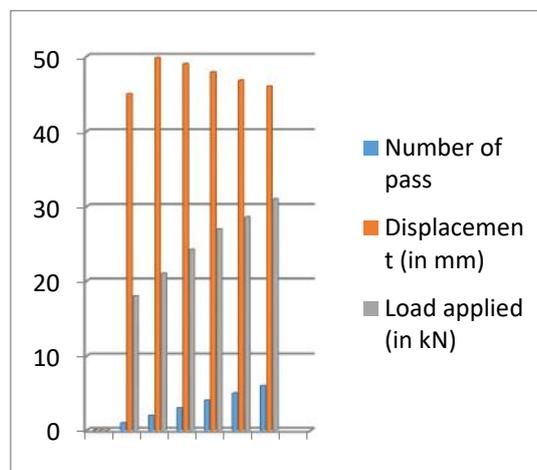
Figure-5: Graph showing variation of load and displacement after various pass
