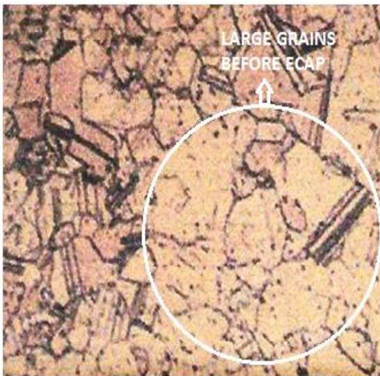
Figure-6: Microstructure of specimen
