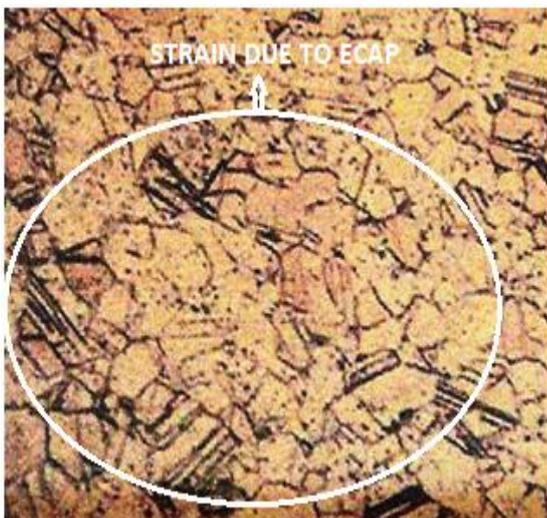
Figure-8: Microstructure after four passes
