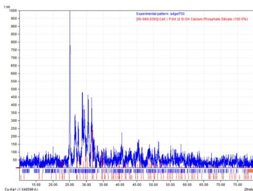
**Fig 3. XRD results of Bioglass Nanoparticles**
