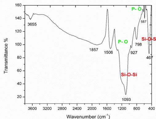
**Fig 4. FTIR Analysis of Bioglass Nanoparticles**
