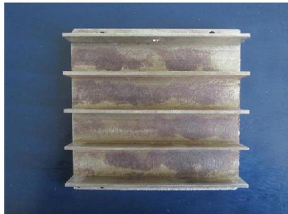
Figure 6. Five-fin sample with 20.5mm fin spacing
