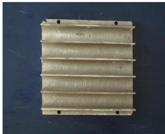
Figure 7. Six-fin sample with 16mm fin spacing
