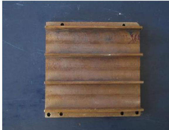
Figure 5. Four-fin sample with 28mm fin spacing
