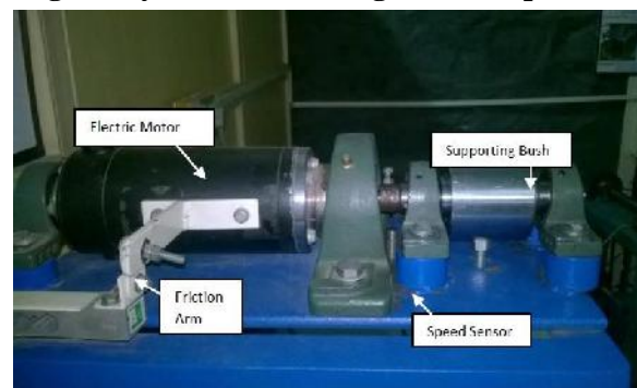
Fig 2. Components of Dry Journal Bearing Setup Close up
