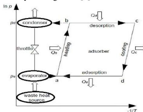
**Fig. 2 Adsorption Cooling Cycle**
