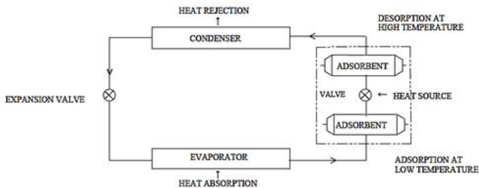
**Fig. 1 Block Diagram of Adsorption Cooling Cycle**
