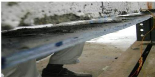
**Fig. 9** Failure mode of beam strengthened with anti-symmetric cross-ply laminate
