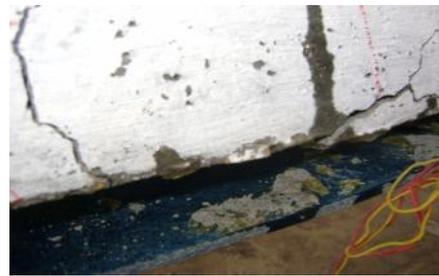
**Fig. 10** Failure mode of beam strengthened with anti-symmetric angle-ply laminate
