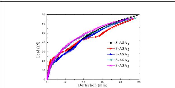
**Fig. 14** Load-deflection behaviour of beams strengthened with anti-symmetric angle-ply laminate
