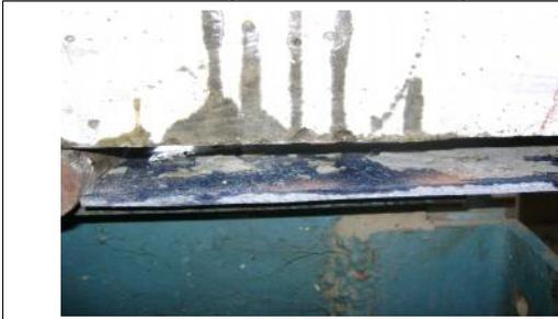
**Fig. 7** Failure mode of beam strengthened with symmetric cross-ply laminate
