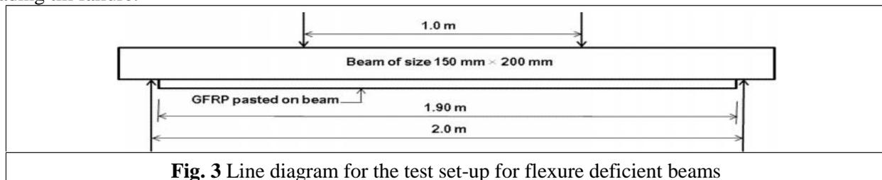
**Fig. 3** Line diagram for the test set-up for flexure deficient beams
