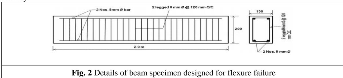
Fig. 2 Details of beam specimen designed for flexure failure
