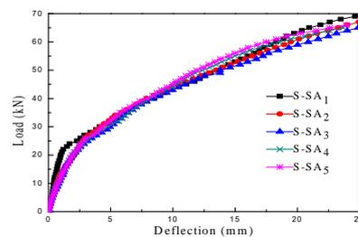
**Fig. 12** Load-deflection behaviour of beams strengthened with symmetric angle-ply laminate
