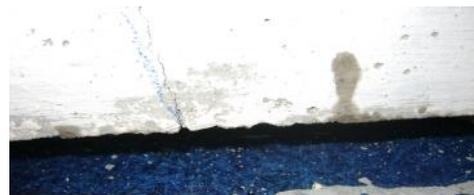
**Fig. 8** Failure mode of beam strengthened with symmetric angle-ply laminate
