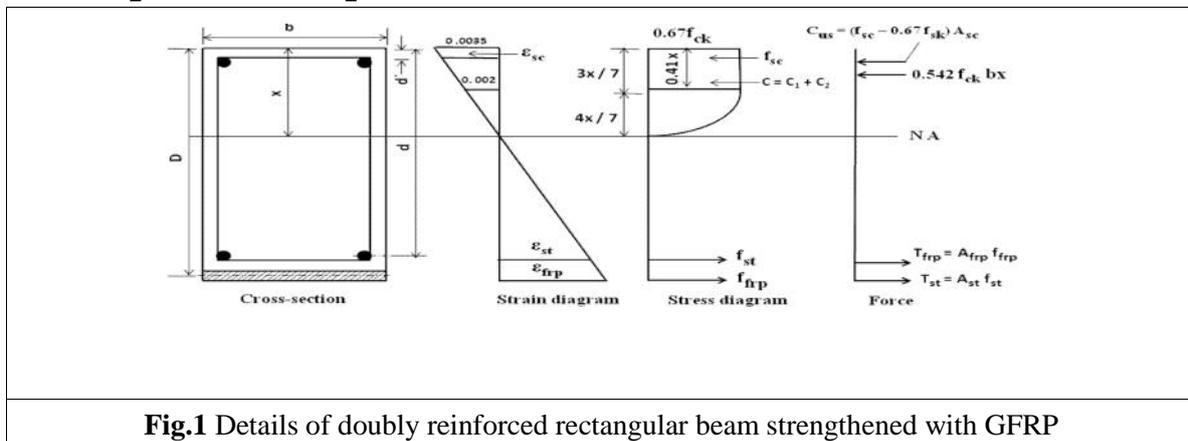
**Fig.1** Details of doubly reinforced rectangular beam strengthened with GFRP
