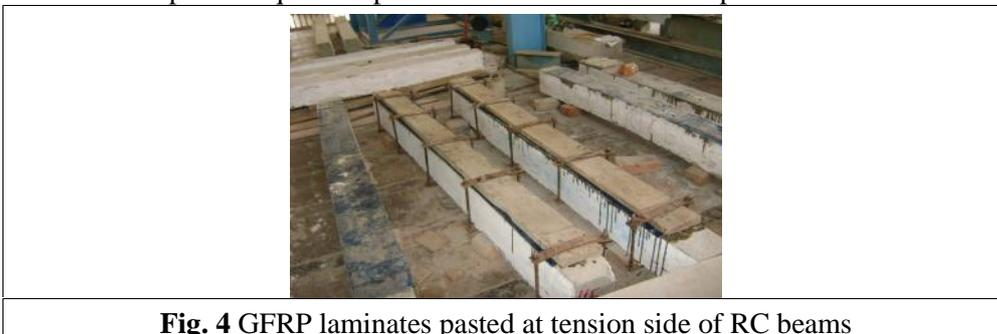
**Fig. 4** GFRP laminates pasted at tension side of RC beams
