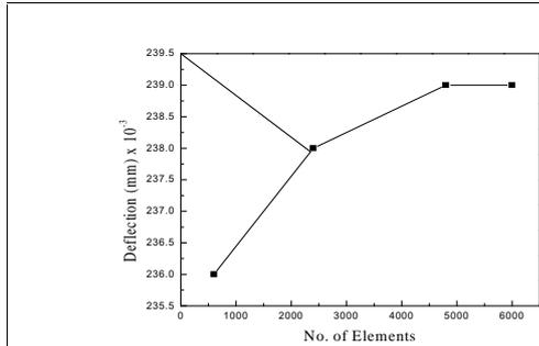
**Fig. 17** Convergence study: displacement at mid-span of beam
