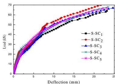
**Fig. 11** Load-deflection behaviour of beams strengthened with symmetric cross-ply laminate
