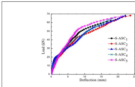
**Fig. 13** Load-deflection behaviour of beams strengthened with anti-symmetric cross-ply laminate
