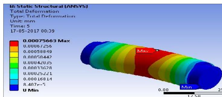
**Fig. 10 Negligible deformation pin**
