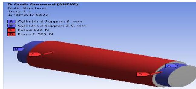
**Fig. 7 Boundary condition for Pin**
