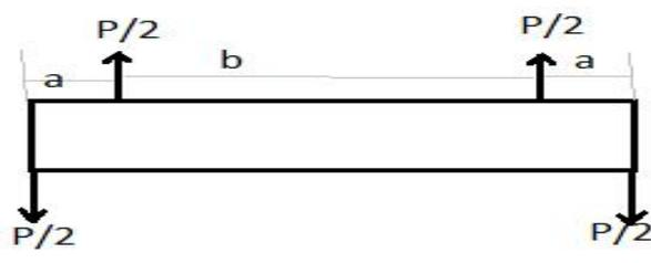
**Fig. 6 Loading Diagram for Pin**
