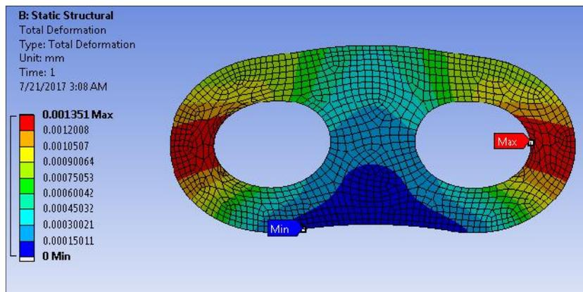
**Fig. 5 Negligible deformation for chain linkage**
