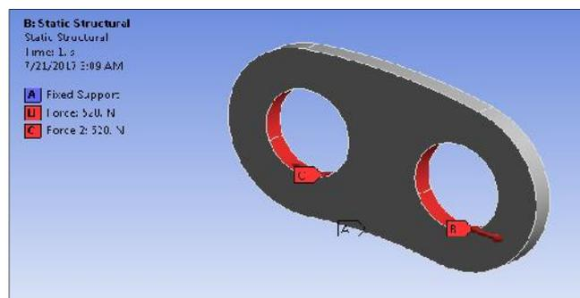
**Fig. 3 Boundary Conditions Applied On Chain Linkage**
