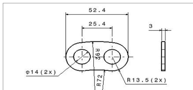
**Fig. 2 2D Drawing of chain linkage**
