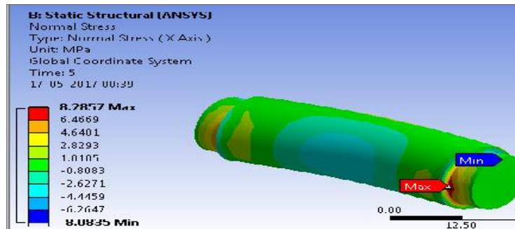
**Fig. 9 Normal Stress for Pin**
