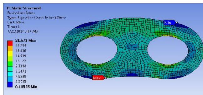
**Fig. 4 Von-Mises stress results for chain linkage**
