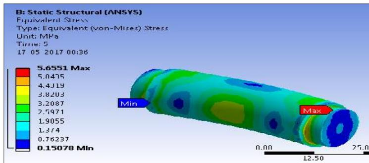
**Fig. 8 Von-Mises Stress Results for Pin**
