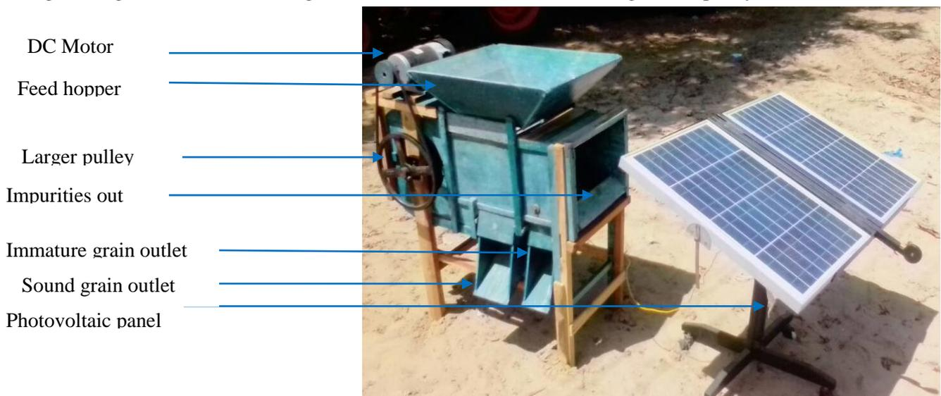
Figure 1. Photovoltaic power operated winnower
