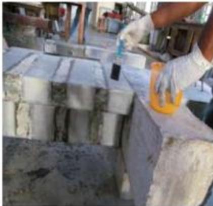
**Fig. 4 Application of epoxy and hardener on the beam**
