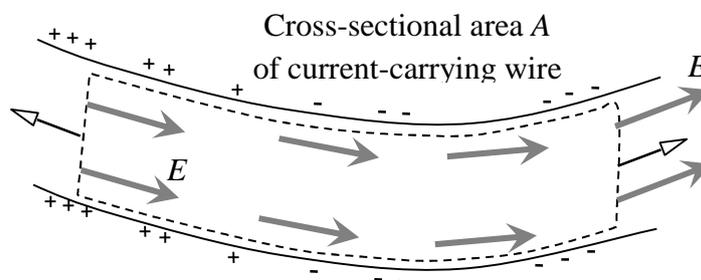
**Fig. 3** In the steady-state, excess charges arrange themselves on the surface of such a wire so that the electric field  $E$  has the same magnitude at different locations along the wire, and is everywhere parallel to the wire. The dashed tube-shaped Gaussian surface nearly fills the wire.
